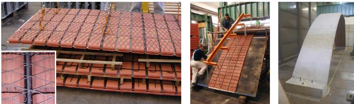
**Figure 2 – Construction of the reinforced brick masonry shell in the laboratory: general view and detail of the semi-prefabricated sheets (left); assembling the shell (centre); view of the shell after casting (right)**
