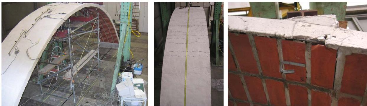
**Figure 9 – Shell before testing (left); crack pattern at the hinge opposite to the loading position, after the test (centre); shell intrados at the loading position, after the test (right)**
