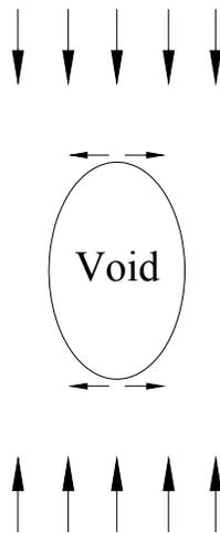
**Figure 2-Tension Is Generated As Compressive Stress Flows Around a Void**
