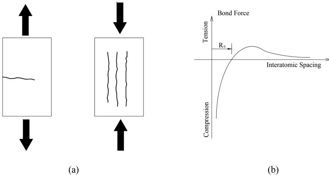
**Figure 1-(a) Uniaxial Tensile Failure with a Single Crack Perpendicular to the Tension and Compressive Failure with Multiple Cracks Parallel to the Compression
