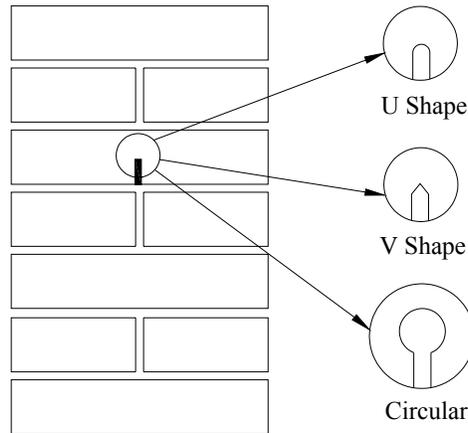
**Figure 4-Different Shapes of Crack Tip**
