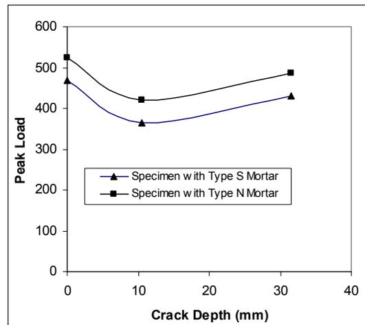
**Figure 10-Peak Load versus Crack Depth**
