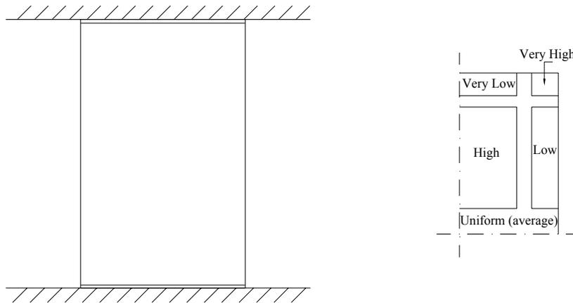
**Figure 5 – Vertical Stress Distributions in Testing Machine**
