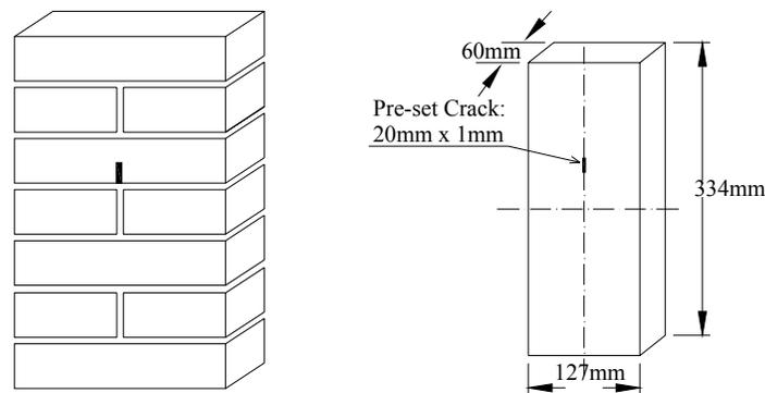
Figure 3 –Specimens with the Pre-set Cracks
