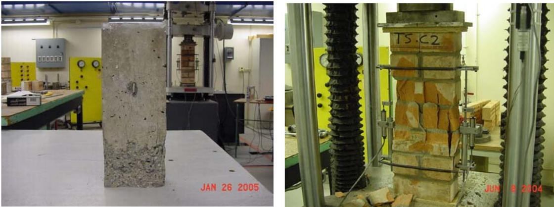
**Figure 7 – Multiple Cracks in Specimens with U and V Shaped Crack Tips**
