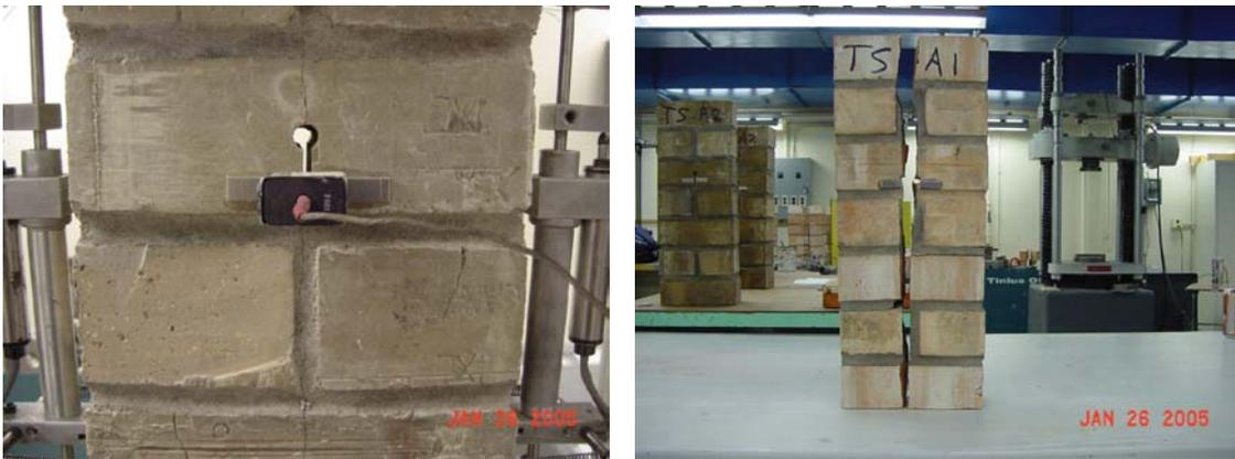
**Figure 8 – Crack with Circular Tip in a Specimen, and the Failed Specimen**
