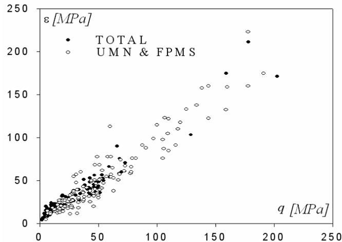
**Figure 5 - Correlation between  $\varepsilon$  and  $q$  [after [3]: for 252 different rock materials]**
