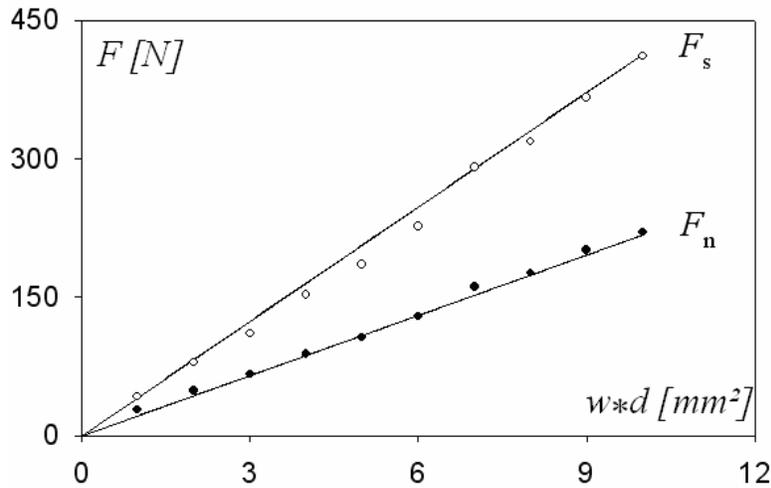
**Figure 3 - Evolution of  $F_s$  and  $F_n$  with  $w*d$  [after (3):  $w = 10\text{mm}$ , *Lens limestone*]**
