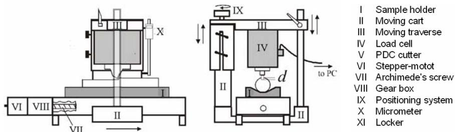
**Figure 2 - Conceptual sketch of the testing device**
