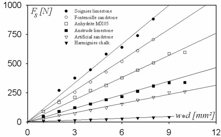
**Figure 4 - Evolution of  $F_s$  with  $w*d$  [after [3]:  $w = 10\text{mm}$ , 6 different rock materials]**
