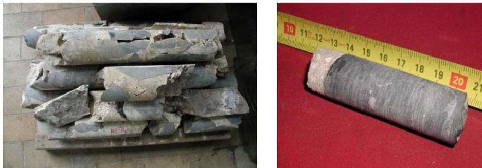
**Figure 8 - Cores removed out of the foundation - normal (left) and small diameter (right)**
