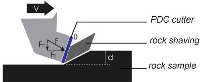
**Figure 1 - Scratching test setup**
