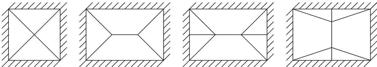
**Figure 1 - Failure Lines and Crack Patterns for Solid Walls Supported on Four Edges**
