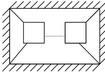
**Figure 6 - Critical Failure Line Pattern for Multiple Small Window Openings**
