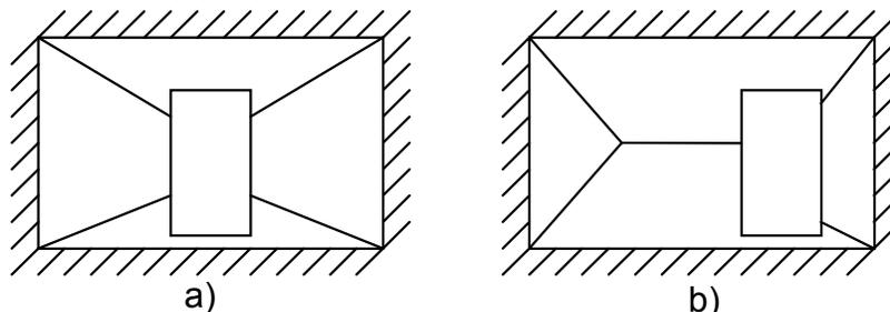
**Figure 7 - Door Centred in Wall Panel and 1.2 m Off-Centre in Wall Panel**
