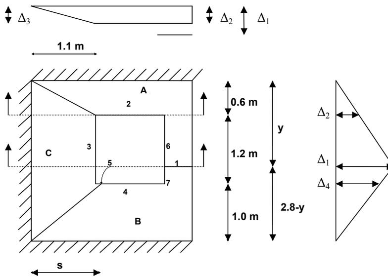
**Figure 3 - Failure Lines for a Wall Supported along Three Edges and Containing a Window**
