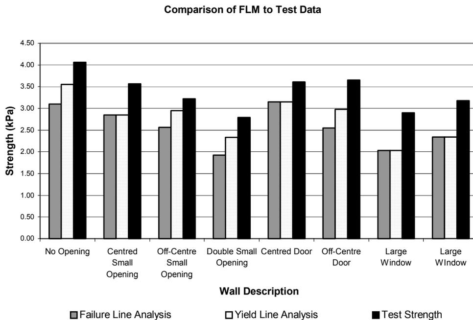
**Figure 9 - The Failure Line Method Compared to Yield Line Analysis and Test Data**
