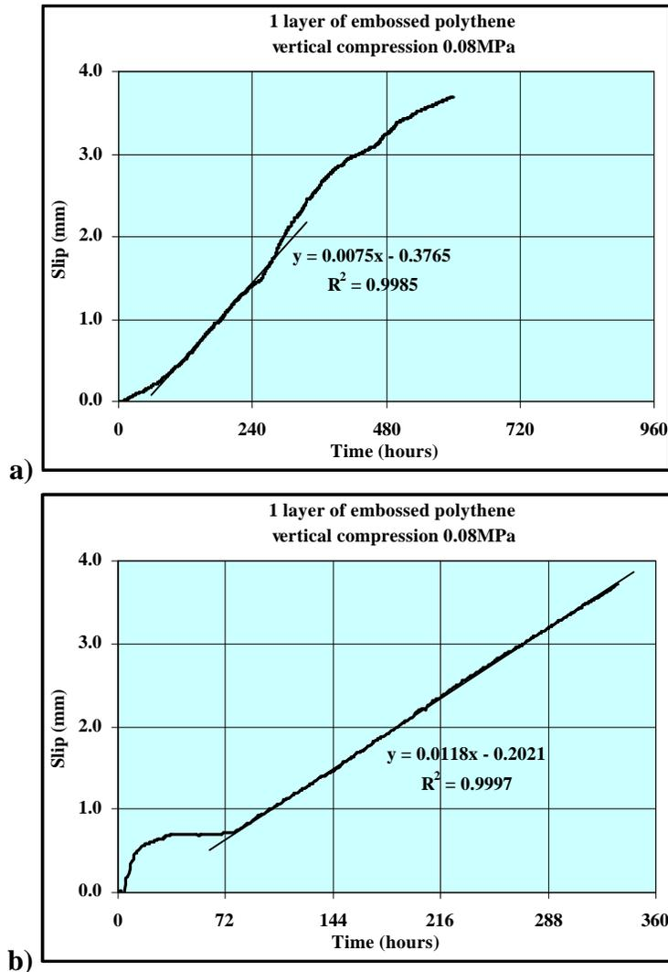
**Figure 5 – Typical Slip Evolution Curves from
