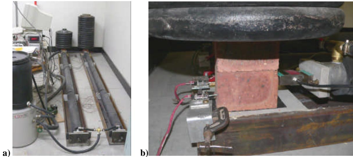
**Figure 3 - Instrumentation Set Up: a) Testing rig; b) Specimen being tested**
