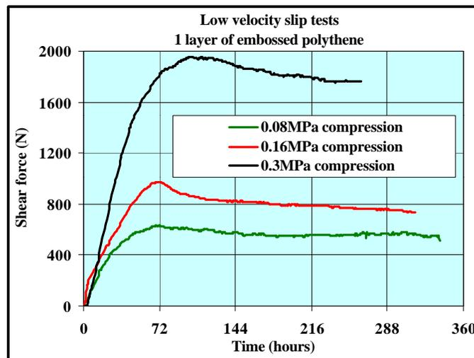
**Figure 6 – Shear Force Evolution Curves**
