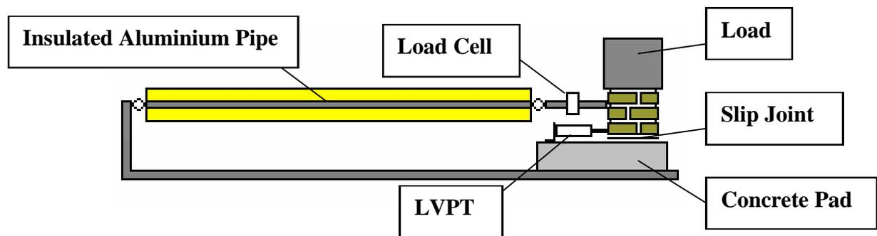
**Figure 2 - Schematic Rig Configuration for Low Velocity Slip Tests**
