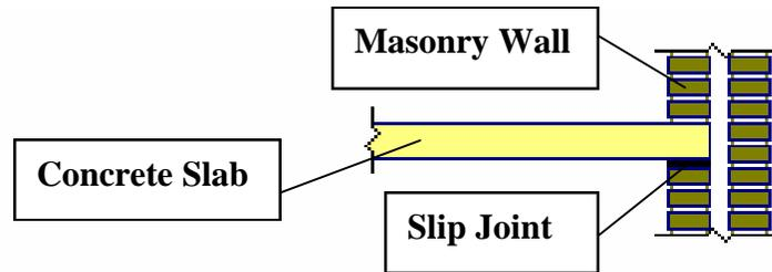
**Figure 1 - Slip Joint in Load-Bearing Masonry Wall**
