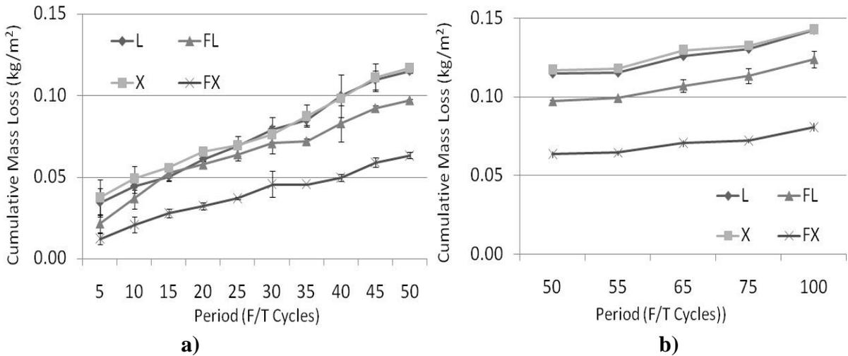
**Figure 6: Average Cumulative Mass in 3% NaCl Solution a) First 50 Cycles b) Last 50 Cycles**
