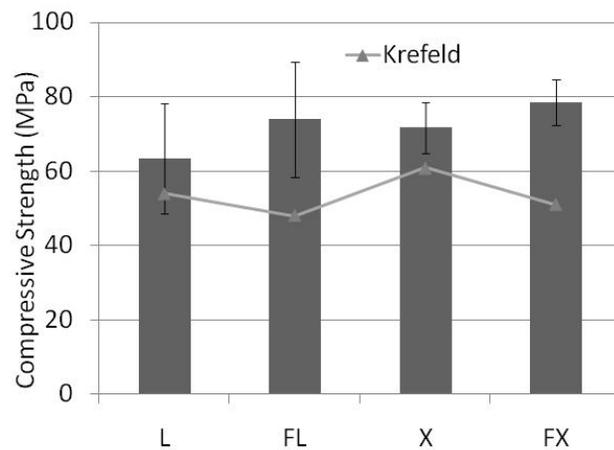
**Figure 1: Average Compressive Strength and Aspect Ratio Adjustment**
