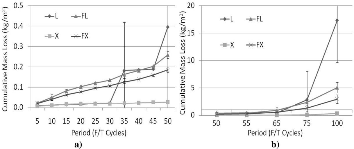
**Figure 5: Average Cumulative Mass Loss in Water a) First 50 Cycles b) Last 50 Cycles**
