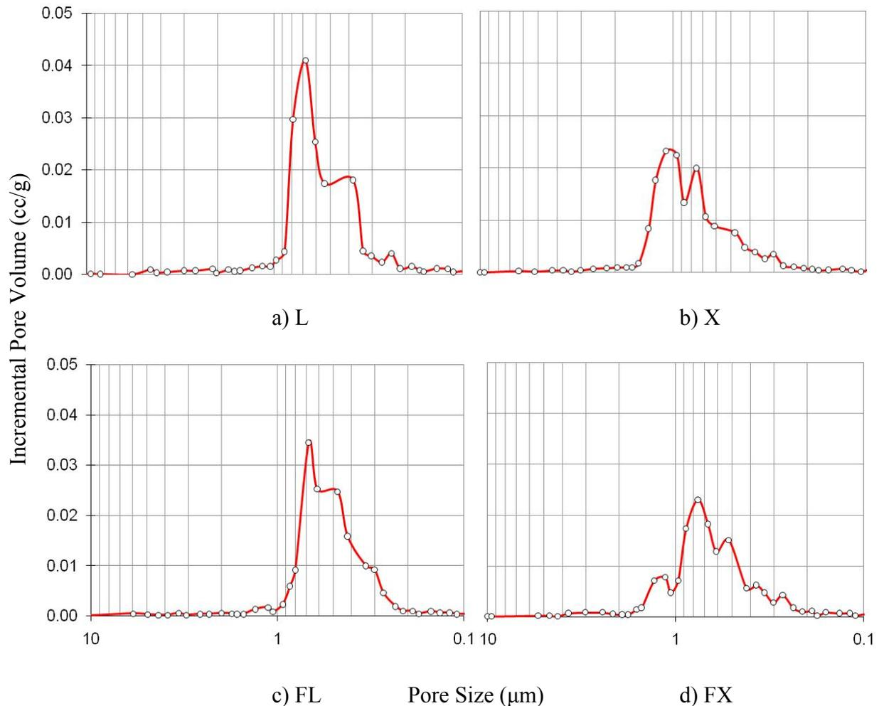
**Figure 7: Pore Size Distribution of Specimens a) L, b) X, c) FL, d) FX by MIP**
