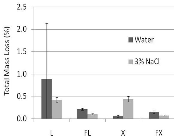
**Figure 8: Percent Mass Loss at 50 Cycles of Freeze-Thaw Testing in Water and 3% NaCl Solution**
