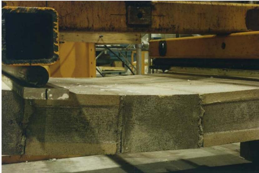
a) Large Rotation and Opening of Cracks for Reinforced Walls
