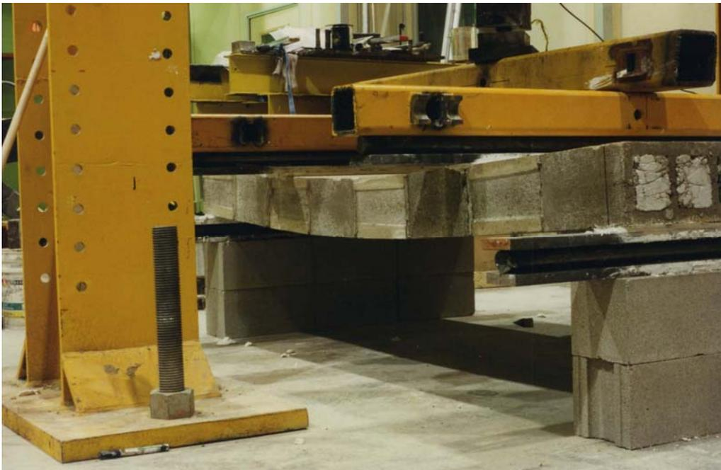
b) Deflection of Reinforced and Fully Grouted Wall
