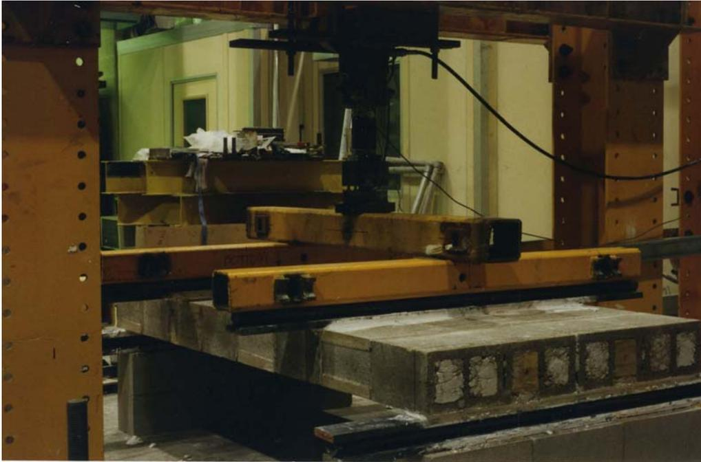
a) Two Point Loading at Quarter Points of Span
