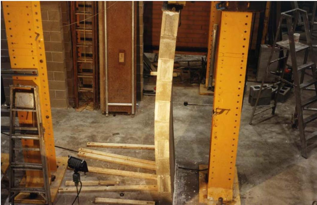
b) Side Elevation Showing Deflection Near Failure
