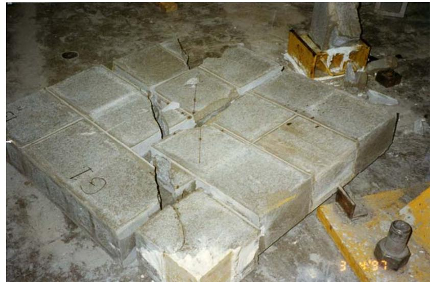
b) Diagonal Crack Pattern
