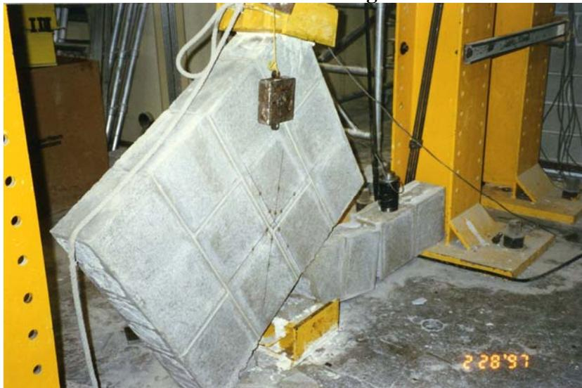
a) Head Joint Failure Pattern
