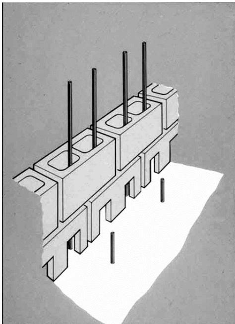
**Figure 4: Reinforced hollow blockwork**
