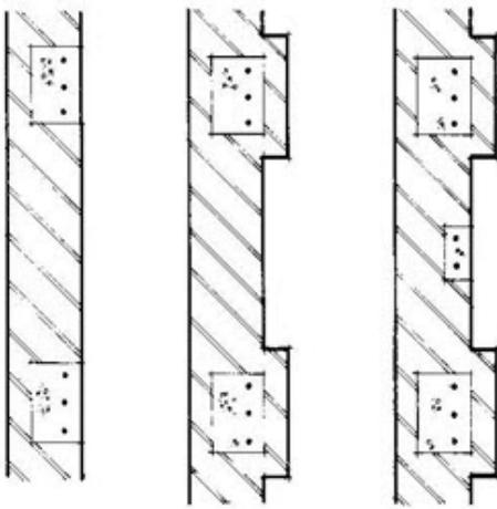
**Figure 2: Plan showing different arrangements of Pocket Type masonry walls**
