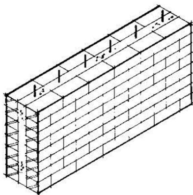
**Figure 1: Grouted cavity masonry.**
