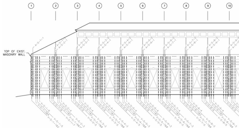
**Figure 5: Portion of reinforcing bar shop drawings showing typical vertical reinforcing location and spacing.**
