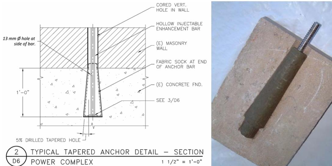
**Figure 6: Left, design detail showing the reverse tapered vertical reinforcing termination. Right, installed taper.**
