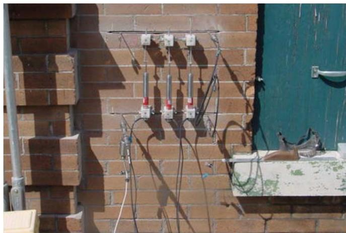
**Figure 4: Flatjack testing at Pump Station 7 to determine existing masonry compressive strength and stiffness.**
