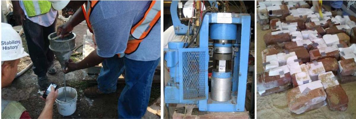
**Figure 9: Left, flow cone testing to verify viscosity of CIF material. Center, compression testing of a hardened CIF sample. Right, brick forms used to cast CIF compression samples.**
