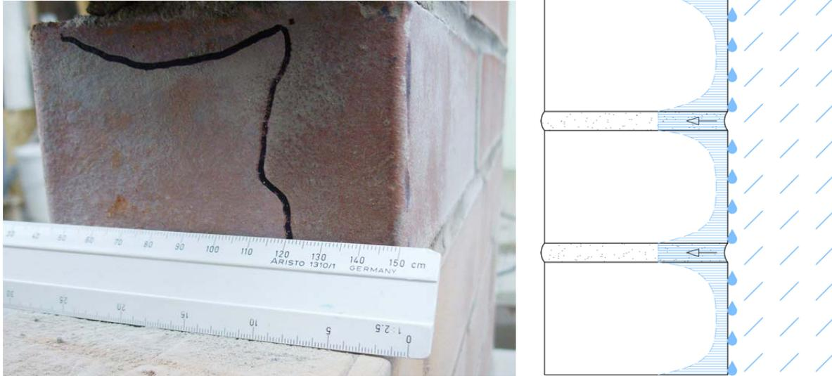
**Figure 6: Test wall No. 2, water penetration after interval spraying of 5 l of applied water (left), schematic of water absorption during driving rain exposition (right)**
