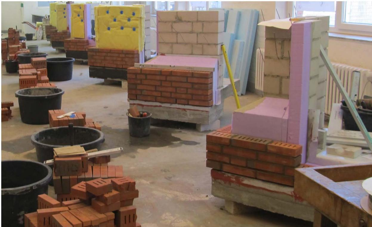
**Figure 8: Test walls to investigate the watertight construction of ground-level door openings considering corners and edges**
