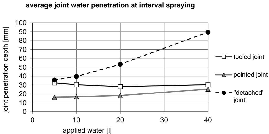
**Figure 4: Average joint penetration depth as a function of amount of applied water**
