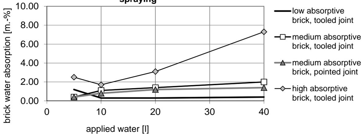
**Figure 7: Brick water absorption after application of a hydrophobing agent as a function of amount of applied water at interval spraying [7]**
