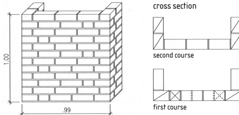
**Figure 3: Laboratory test walls**
