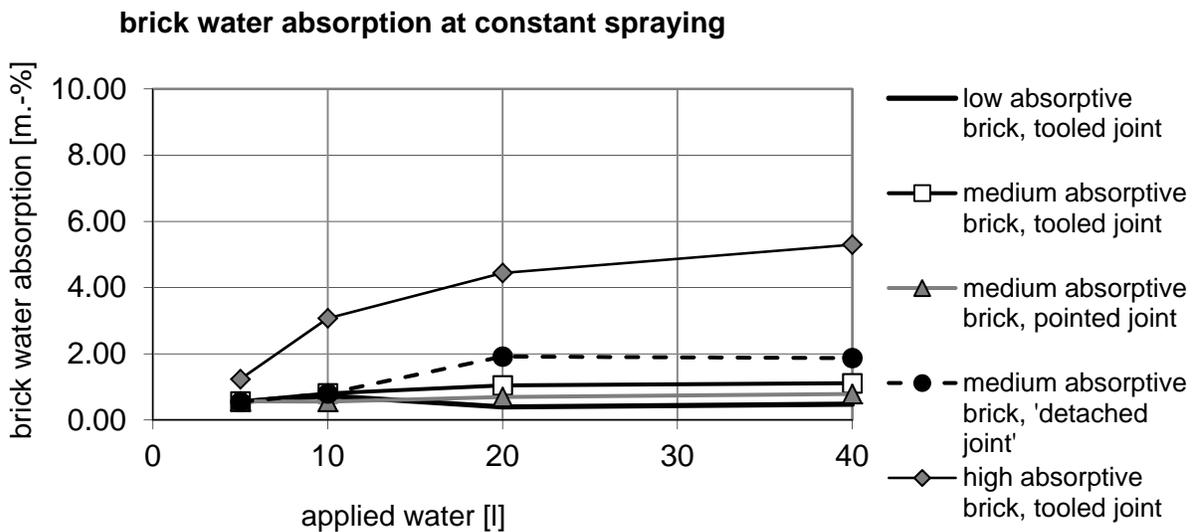
**Figure 5: Brick water absorption as a function of amount of applied water, compared at interval and constant spraying**
