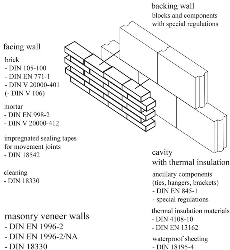
**Figure 1: Masonry veneer walls: principle and referring standards [3]**
