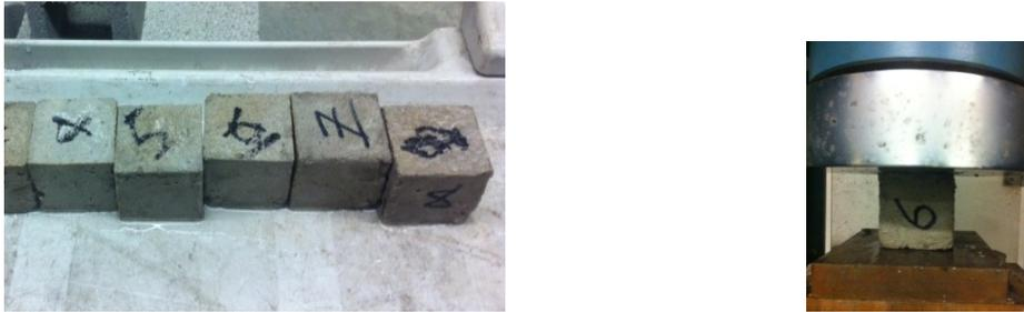
**Figure 3: Axial Compression of Mortar Cubes**
