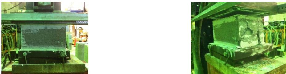
**Figure 2: Axial Compression Test of Masonry Units**
