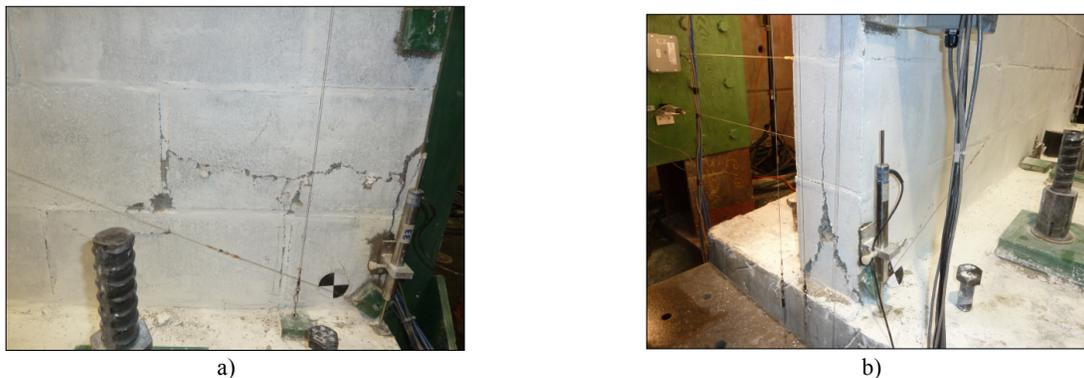
**Figure 7: Cracking at the target displacement  $3\Delta_y$ : a) North toe, and b) South toe**
