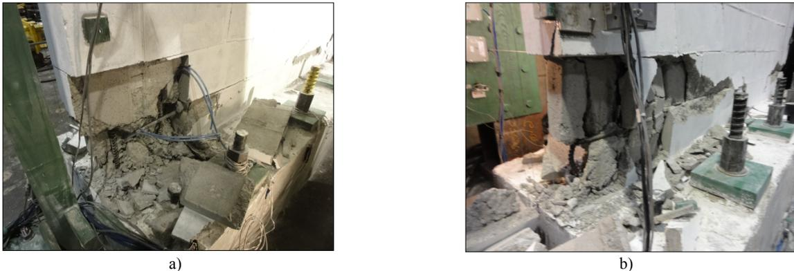
**Figure 9: Specimen failure at the target displacement  $6\Delta_y$ : a) North toe, and b) South toe**
