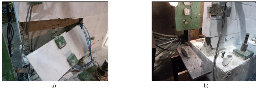
**Figure 8: Specimen damage at the target displacement  $4\Delta_y$ : a) North toe, and b) South toe**
