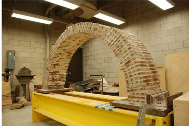
**Figure 1: Brick Arch Specimen – Scale Model of One of the Arches in Brooklyn Bridge**
