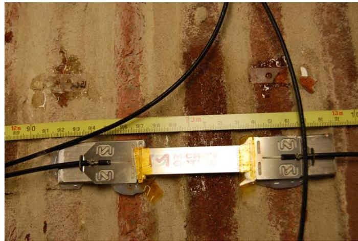
**Figure 4: Glass Fibre Strain Gauges Fabricated by Micron Optics, Inc.**
