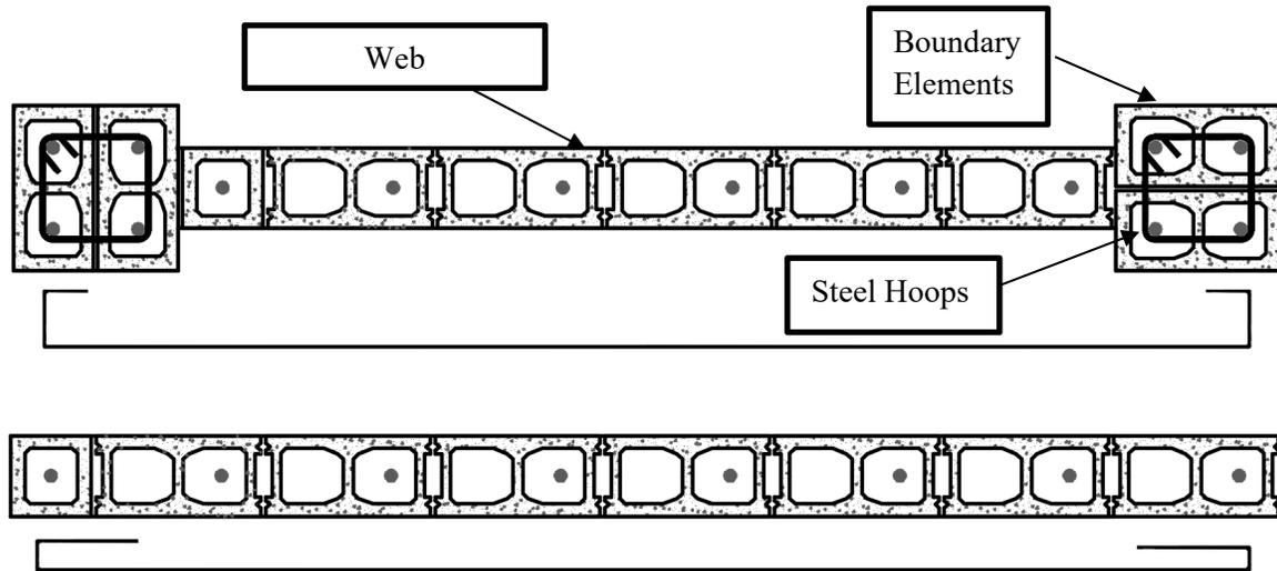
**Figure 1: Reinforcement detailing in BE-walls vs. regular walls**
