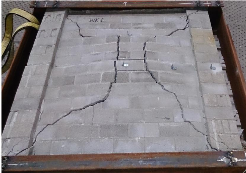
**Figure 5: Failure crack pattern under static loading**
