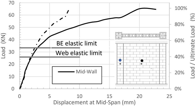
**Figure 4: Mid-span load-displacement curves recorded during static testing**
