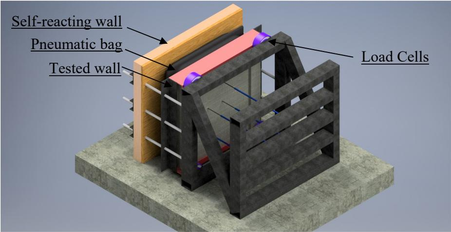
**Figure 3: Schematic of the static test setup**
