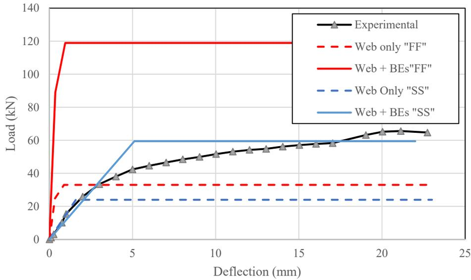
**Figure 6: Comparison of predicted resistance functions (DIF = 1) with data from static testing**
