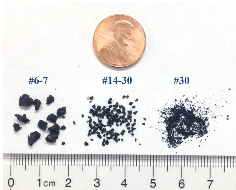
**Figure 1: Different sizes of crumb rubber used in production of RCMUs**
