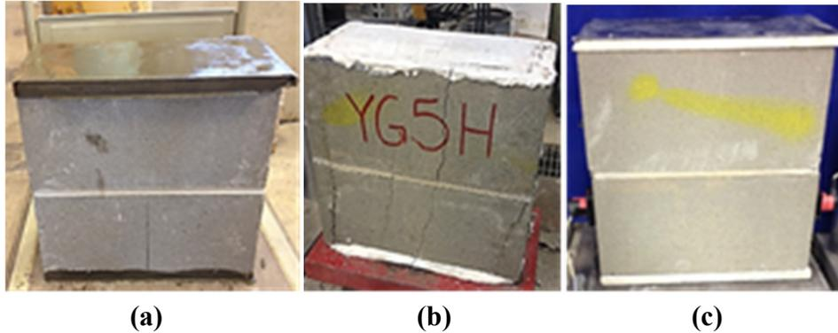
**Figure 2: Different capping types: (a) Sulfur capping layers, (b) Gypsum capping layers and (c) Fibrous composite laminated cap**
