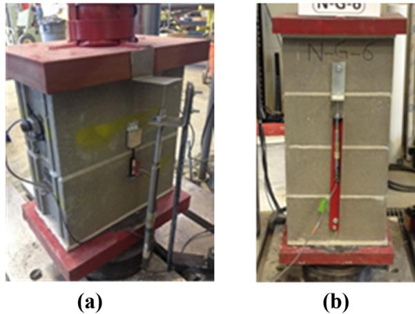
**Figure 4. Displacement measurement instrumentations (a) Two-block high prisms, and (b) Four-block high prisms**
