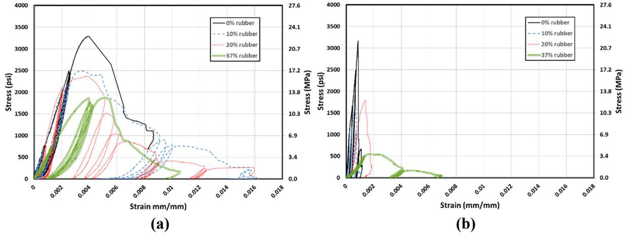
**Figure 8: Stress vs. strain for two blocks height masonry prisms**
