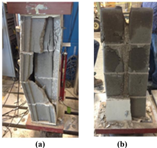
**Figure 7: Failure mechanism for four blocks height prisms with no rubber added. (a) side view (b) front view**
