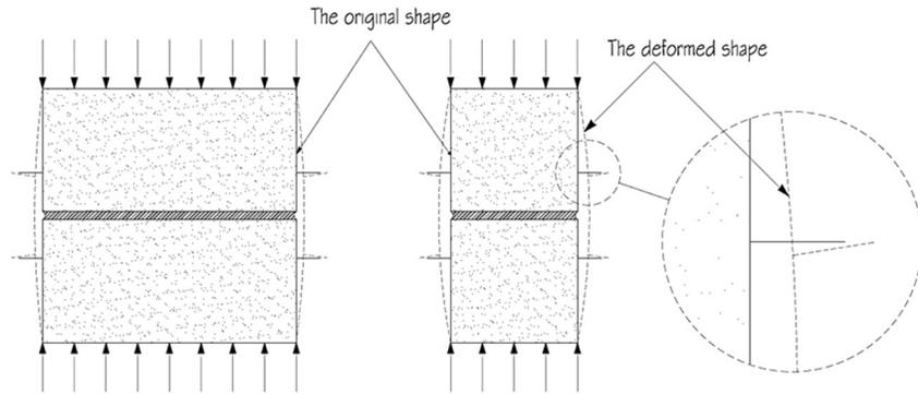
**Figure 5. Effects of bulging on the points at which the strain was measured**
