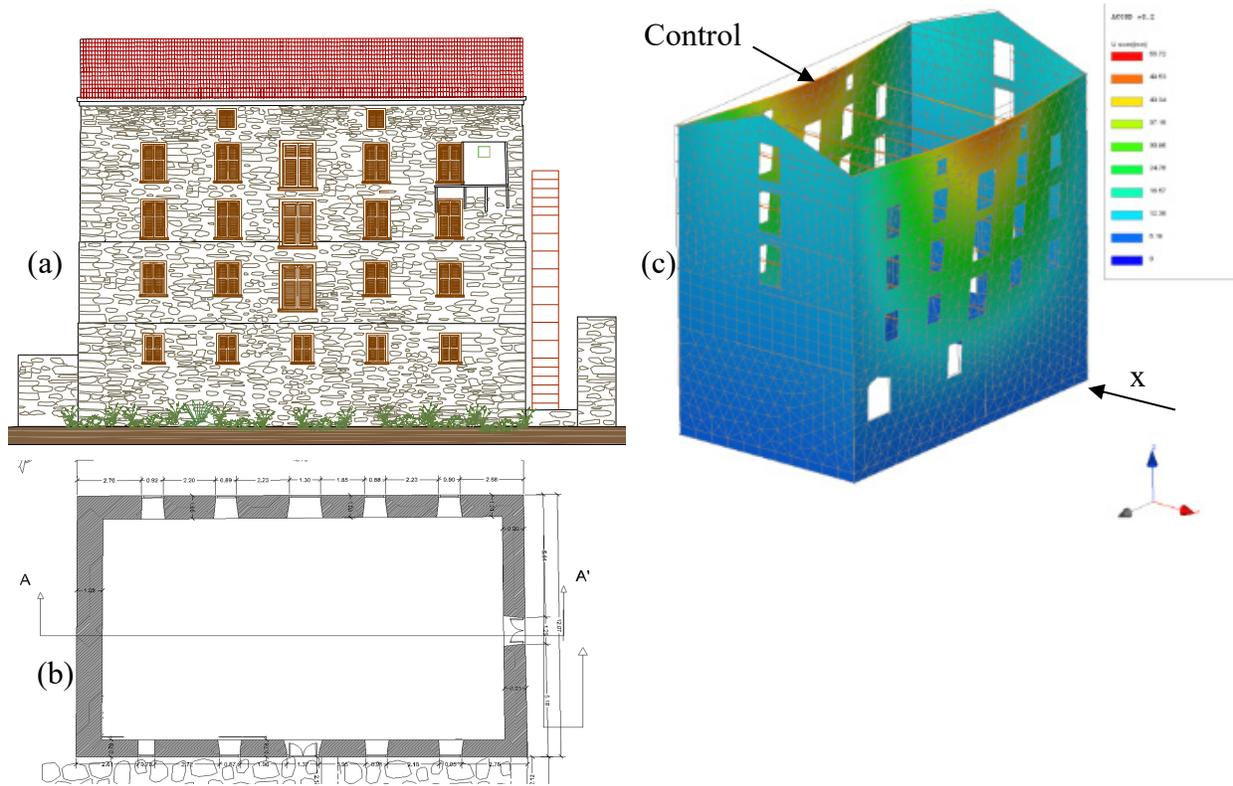
**Figure 1: Water mill in Andros –typical application example analysed according with [2]: (a) elevation and (b) plan view (c) Deformation: flexible diaphragms for seismic action // to the x axis**
