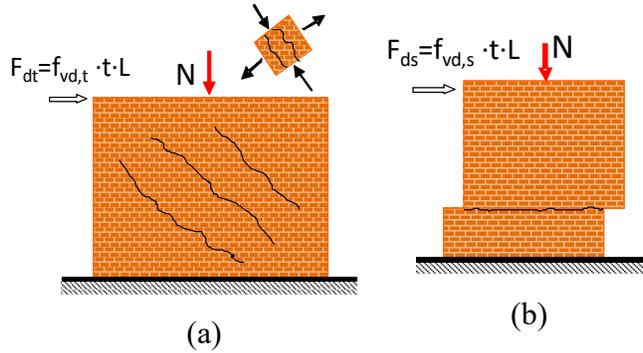
**Figure 4: Shear failure: a) diag. cracking, b) sliding**
