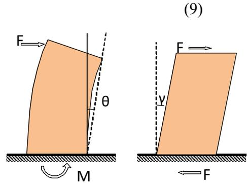
**Figure 7: Wall under in plane force**
