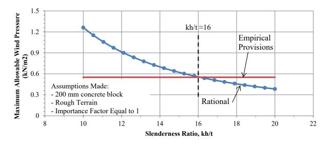
Figure 1: Effect of Slenderness Ratio on the Flexural Strength of walls based on Empirical and Rational Provisions
