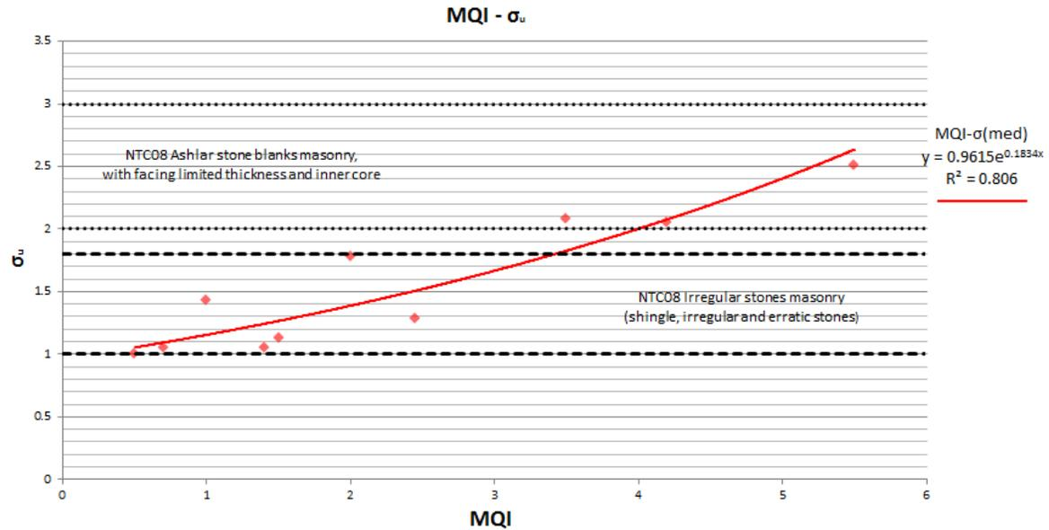
**Figure 6: All masonry types correlation curve**
