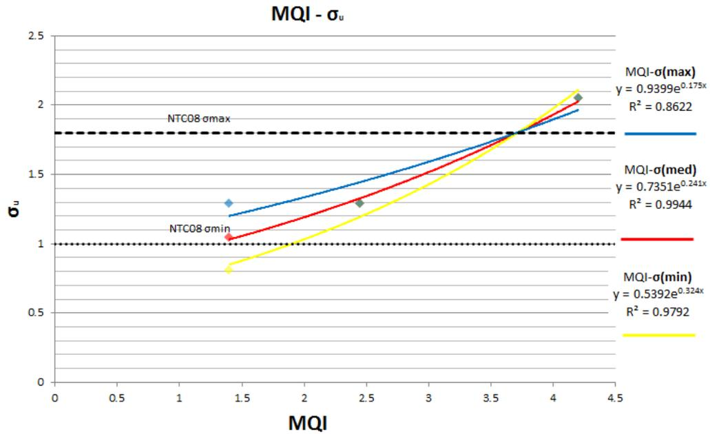
**Figure 4: Irregular stone with brick lines correlation curve**
