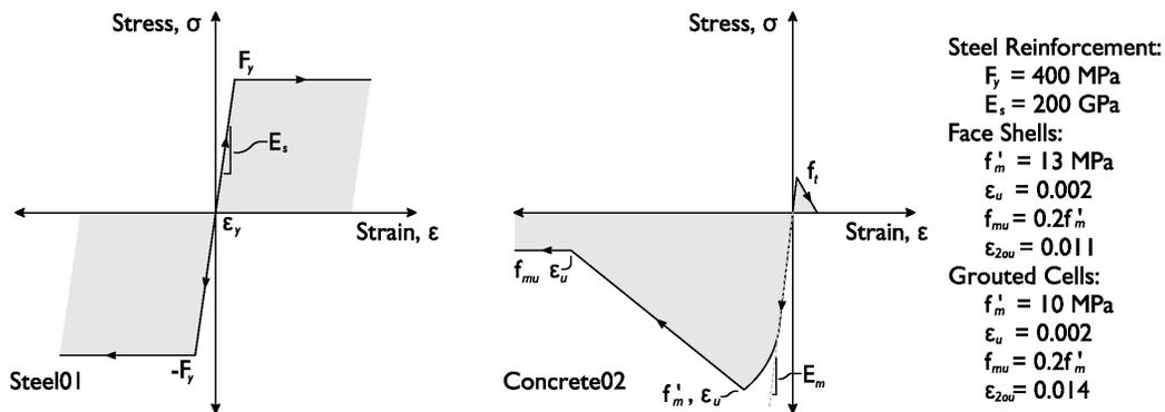
**Figure 4: Material Constitutive Relationships for Steel (left) and Masonry (right)**
