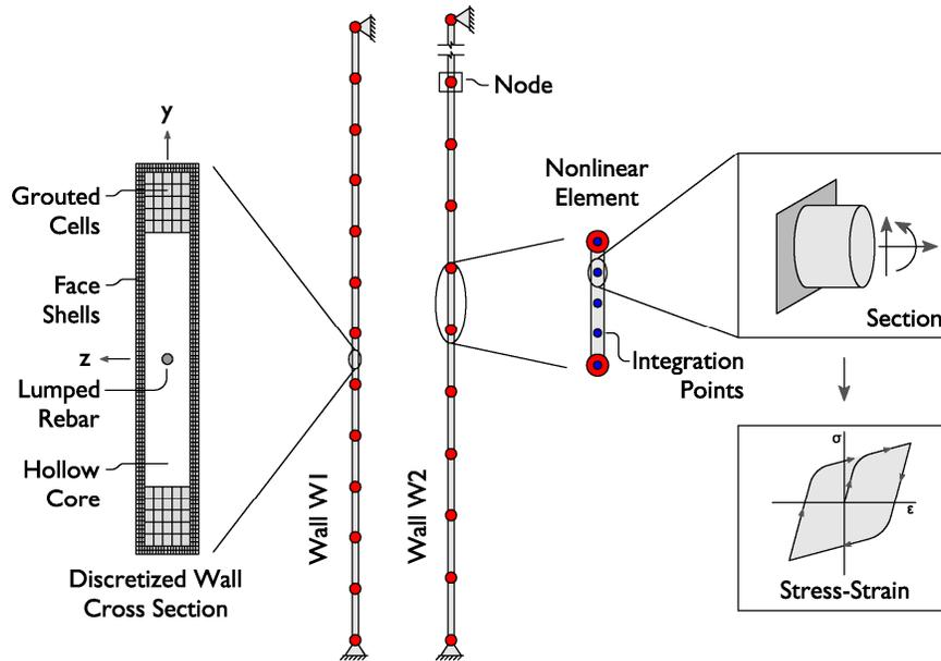
**Figure 3: OpenSees Analytical Model and Fibre Section**
