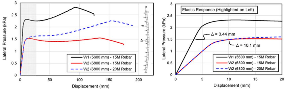
**Figure 5: Lateral Pressure versus Top Displacement Response**
