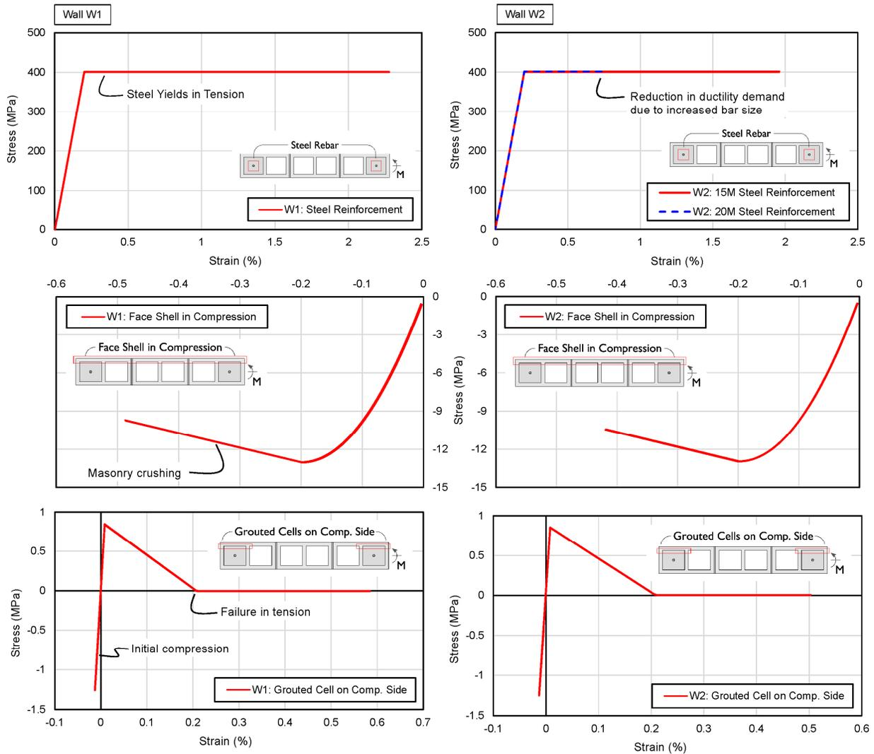
**Figure 6: Stress-strain Response for Walls W1 and W2**
