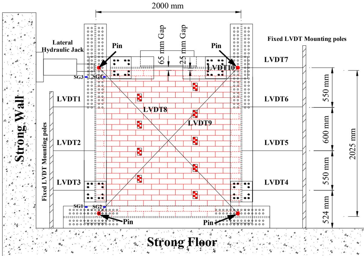
**Figure 3: Experimental Set Up for In-Plane Cyclic Testing of SIM Panels**
