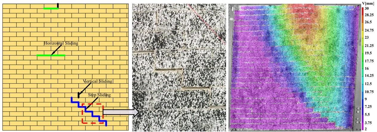
a) Panel 1: SIM Infill Panel with Open Gap
