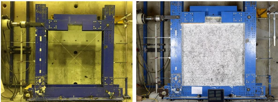
**Figure 6: Photograph of Experimental Setup: Bare Frame Mechanism (left) and Frame Mechanism with Panel Showing Speckle Pattern Applied for DIC (right)**
