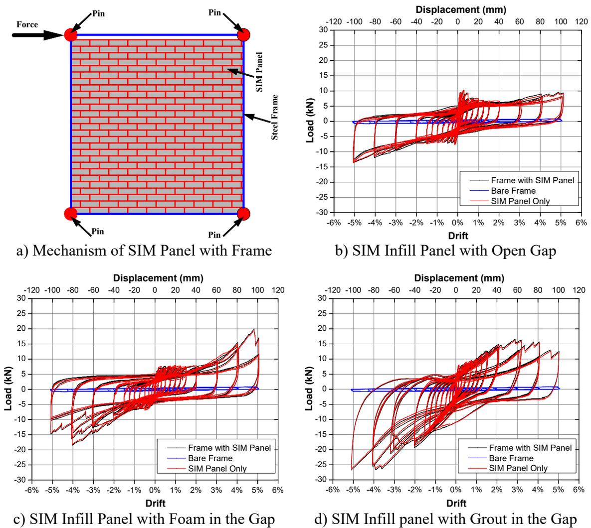
**Figure 8: Overall Structural Response of the SIM panels**
