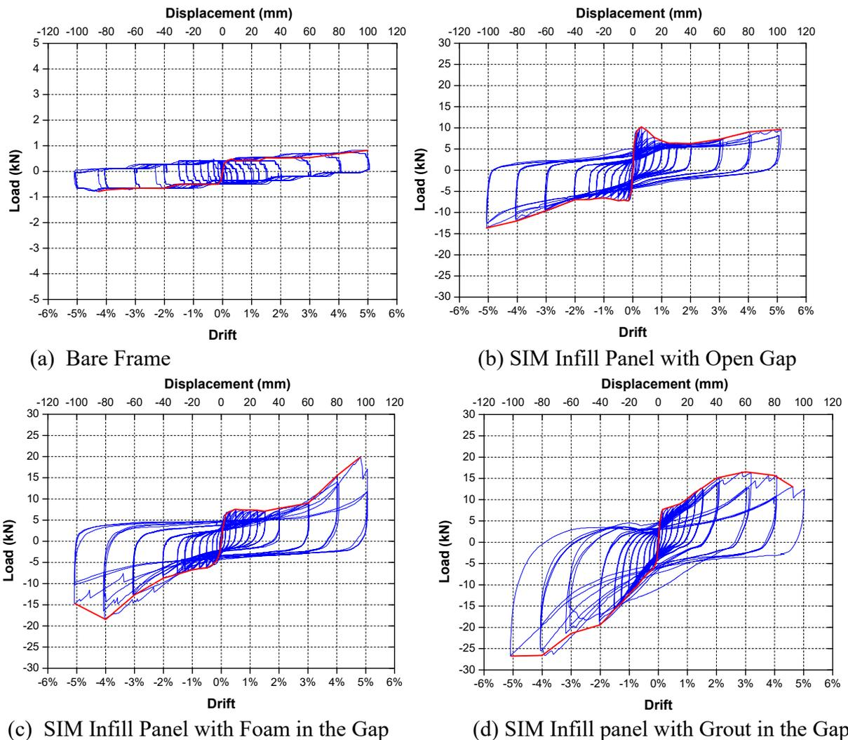
**Figure 7: Force–Displacement Response Hysteresis of the Tested Panels**
