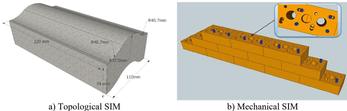
**Figure 2: Types of Semi-Interlocking Masonry (SIM)**
