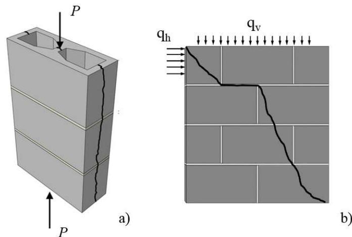
**Figure 1: Typical cracking in HCB masonry by tensile stress a) prism under axial compression, b) wallete under lateral loads**
