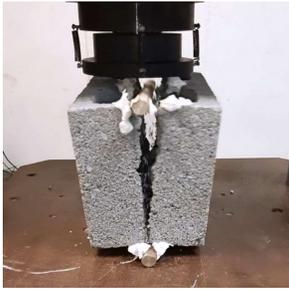
S-3. Splitting test in y-direction
