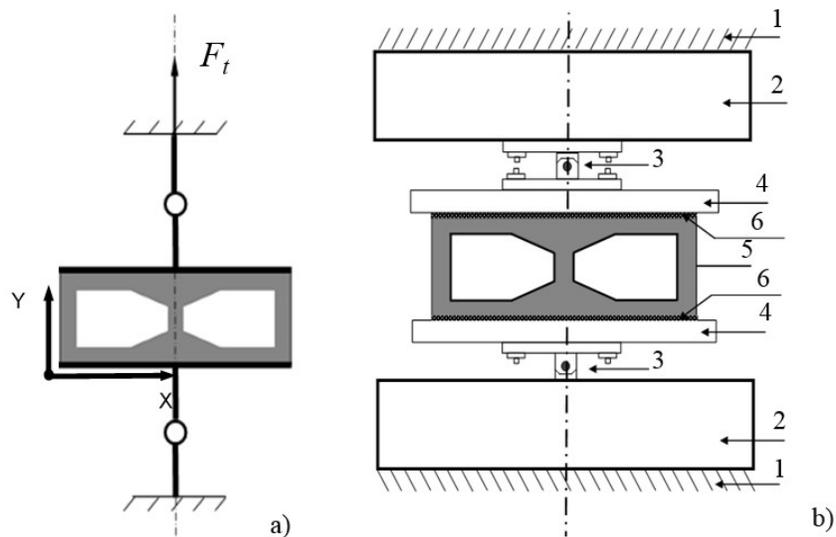
**Figure 5: Test setup for S-5 series: (a) schematic arrangement, (b). Front view. Where: 1. Machine support frame, 2. Upper and lower clamps, 3. Hinged elements for transmitting the load, 4. Plates, 5. Specimen, 6. Epoxy resin**
