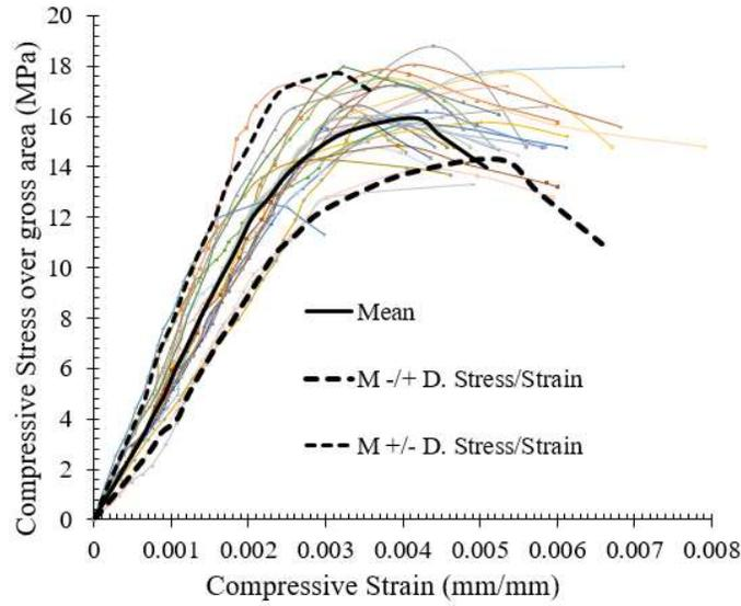
**Figure 6: Experimental axial compression stress-strain relationships ( $\sigma$  vs  $\epsilon$ ) of HCB**
