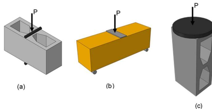
**Figure 2: Indirect tensile tests of masonry units: (a) splitting test, (b) flexure test and, (c) compressive test into the parallel direction to the bed joints**
