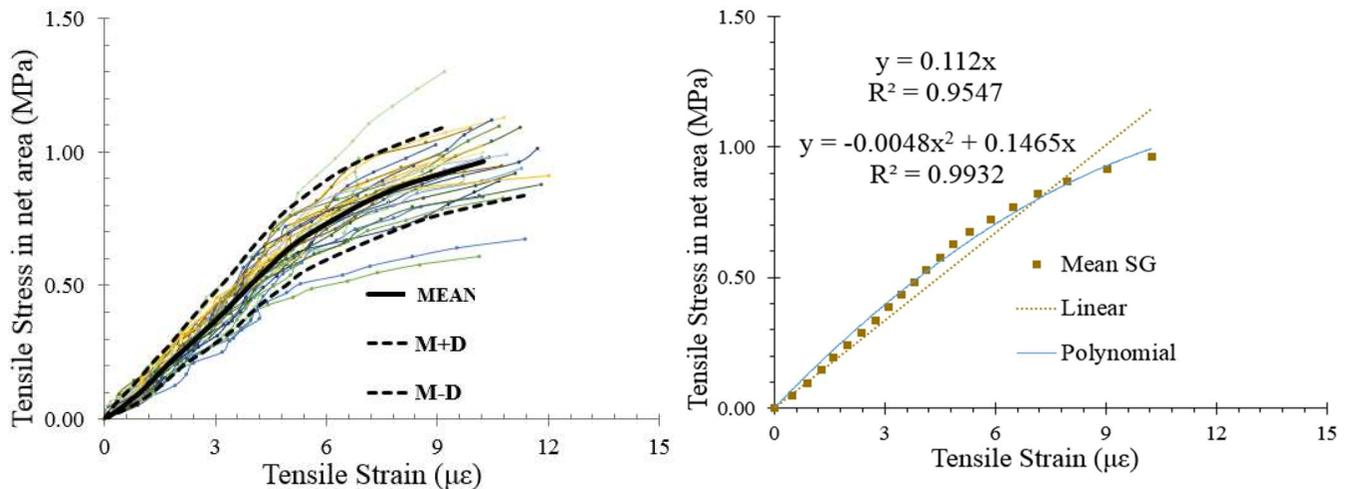
**Figure 8: Stress-strain relationships from the S-5 results**
