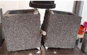
S-2. Splitting test in x-direction
