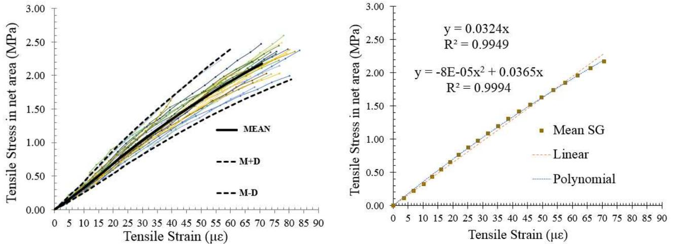
**Figure 7: Stress-strain relationships from the S-4 results**
