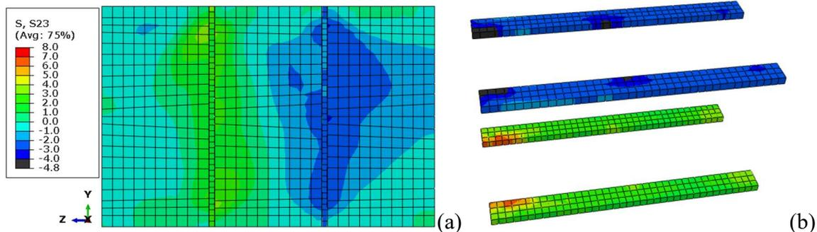
**Figure 3: Shear Stress Distribution of Triplet Test: (a) Entire Specimen; (b) Mortars Only**
