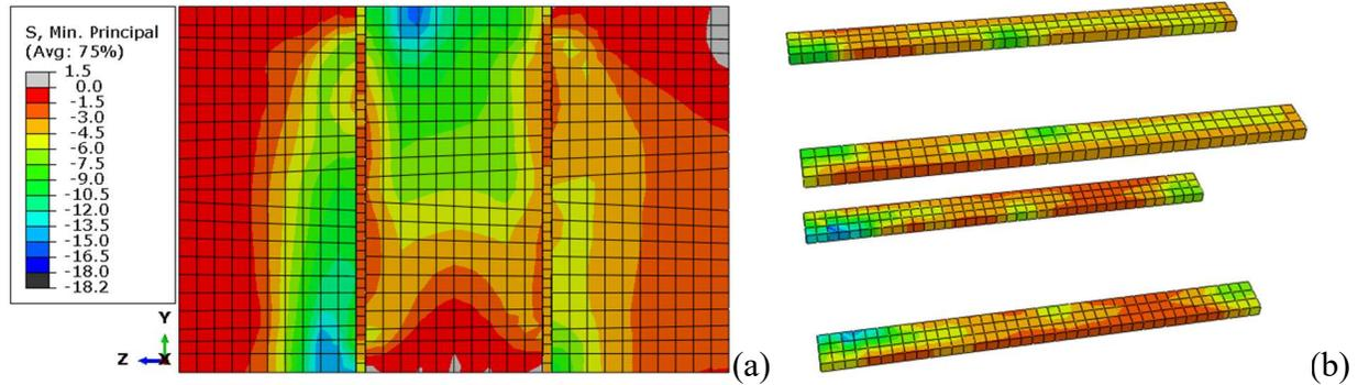
**Figure 4: Minimum Principal Stress Distribution of Triplet Test: (a) Entire Specimen; (b) Mortars Only**
