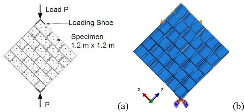
**Figure 2: (a) Diagonal Tension Test; (b) Abaqus Model of Diagonal Tension Test**
