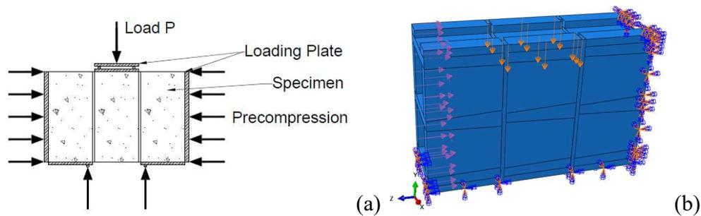
**Figure 1: (a) Triplet Test with Precompression Load; (b) Abaqus Model of Triplet Test**
