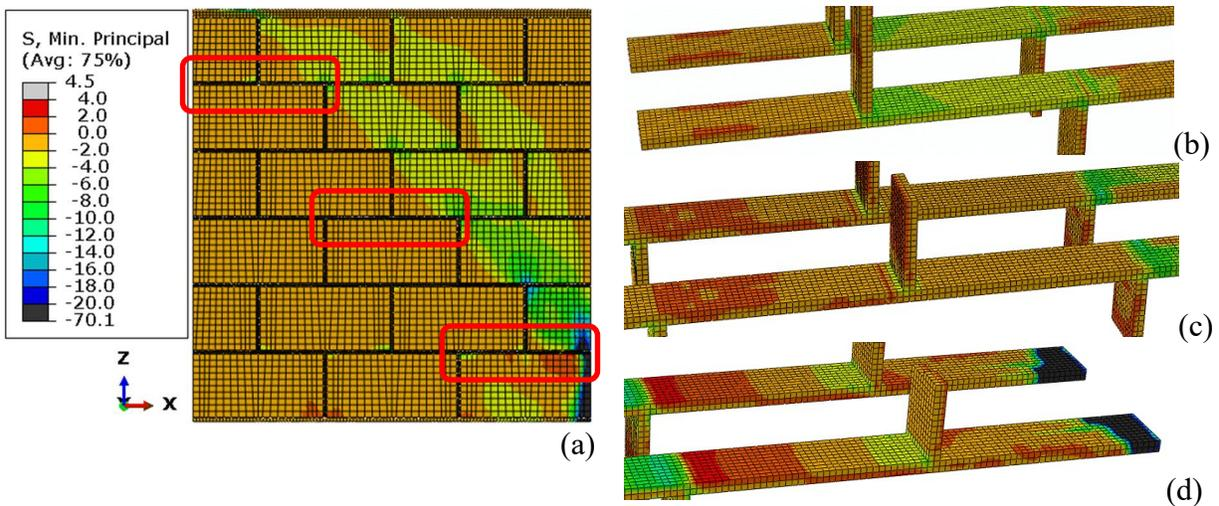
**Figure 8: Minimum Principal Stress Distribution of Wall with Uniform Stress: (a) Entire Specimen; (b) the Top Mortar; (c) the Middle Mortar; (d) the Bottom Mortar**
