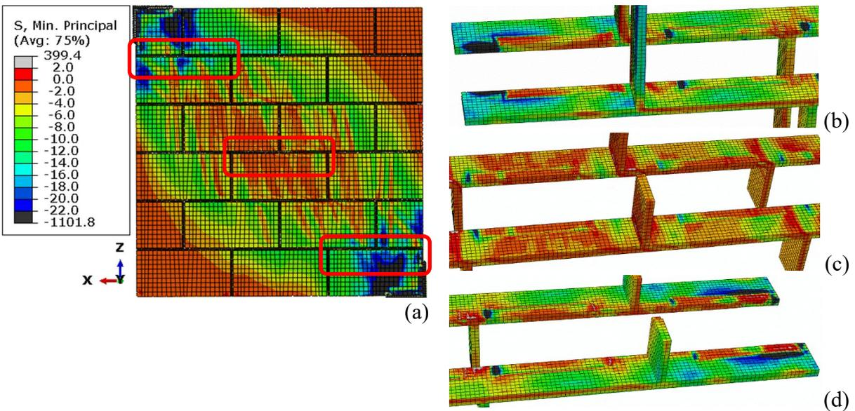
**Figure 6: Minimum Principal Stress Distribution of Rotated Diagonal Tension Test Model: (a) Entire Specimen; (b) the Top Mortar; (c) the Middle Mortar; (d) the Bottom Mortar**
