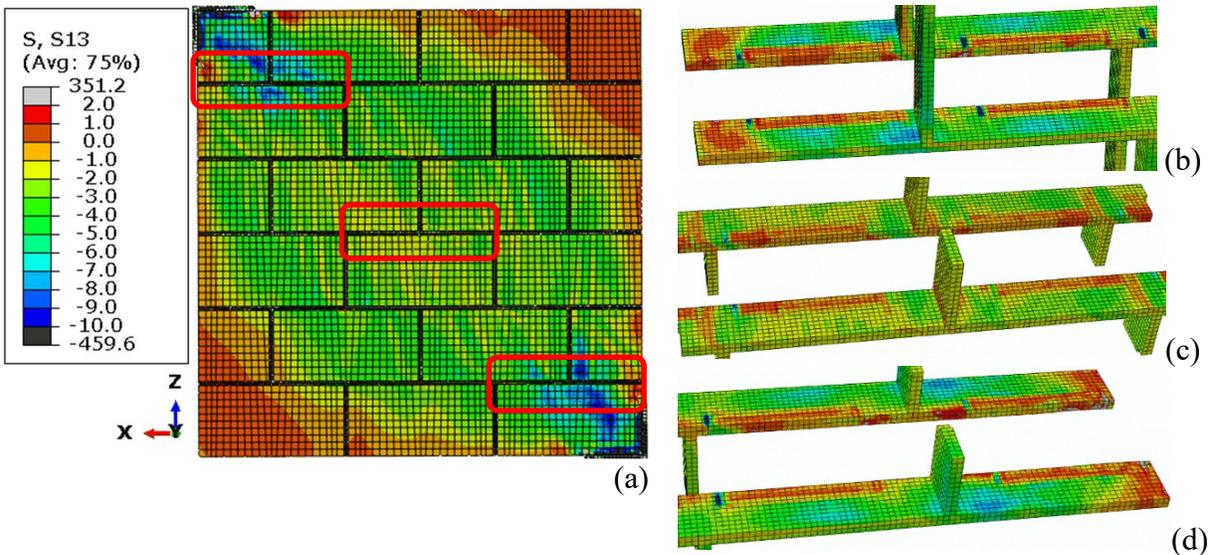
**Figure 5: Shear Stress Distribution of Rotated Diagonal Tension Test Model: (a) Entire Specimen; (b) the Top Mortar; (c) the Middle Mortar; (d) the Bottom Mortar**
