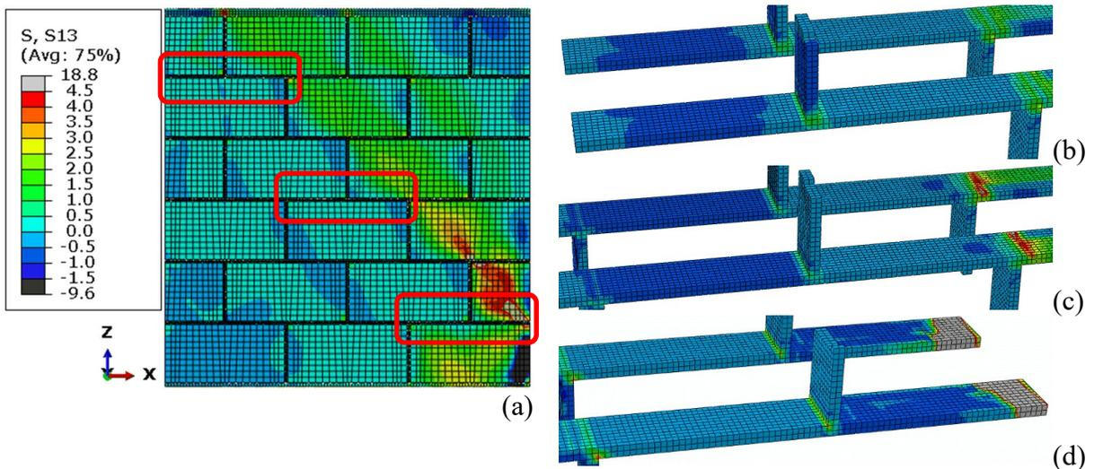
**Figure 7: Shear Stress Distribution of Wall with Uniform Stress: (a) Entire Specimen; (b) the Top Mortar; (c) the Middle Mortar; (d) the Bottom Mortar**
