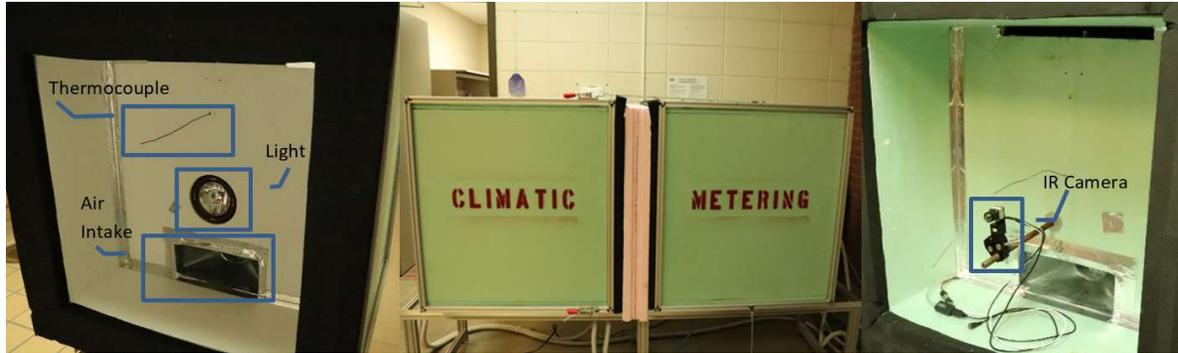
**Figure 1: Small Scale Hot Box climatic (right), exterior, and metering (left) view**
