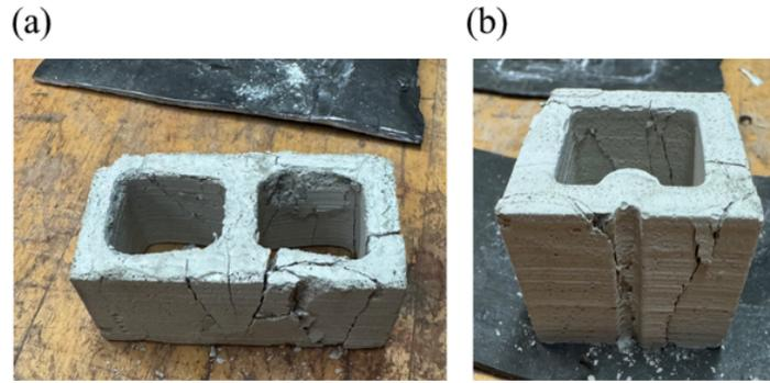
**Figure 5: Specimens after testing: (a) full-size CMU and (b) half-size CMU.**
