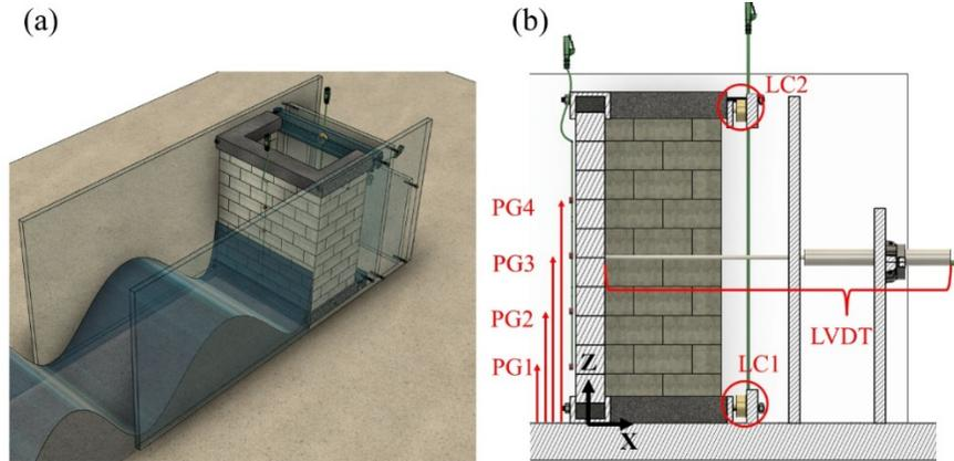
**Figure 9: (a) Orthographic view of the test setup for C - shaped masonry walls. (b) C - shaped masonry wall instrumentation plan with two load cells (LC1 and LC2), one linear variable differential transformer (LVDT), and five pressure gages (PG1-PG4).**
