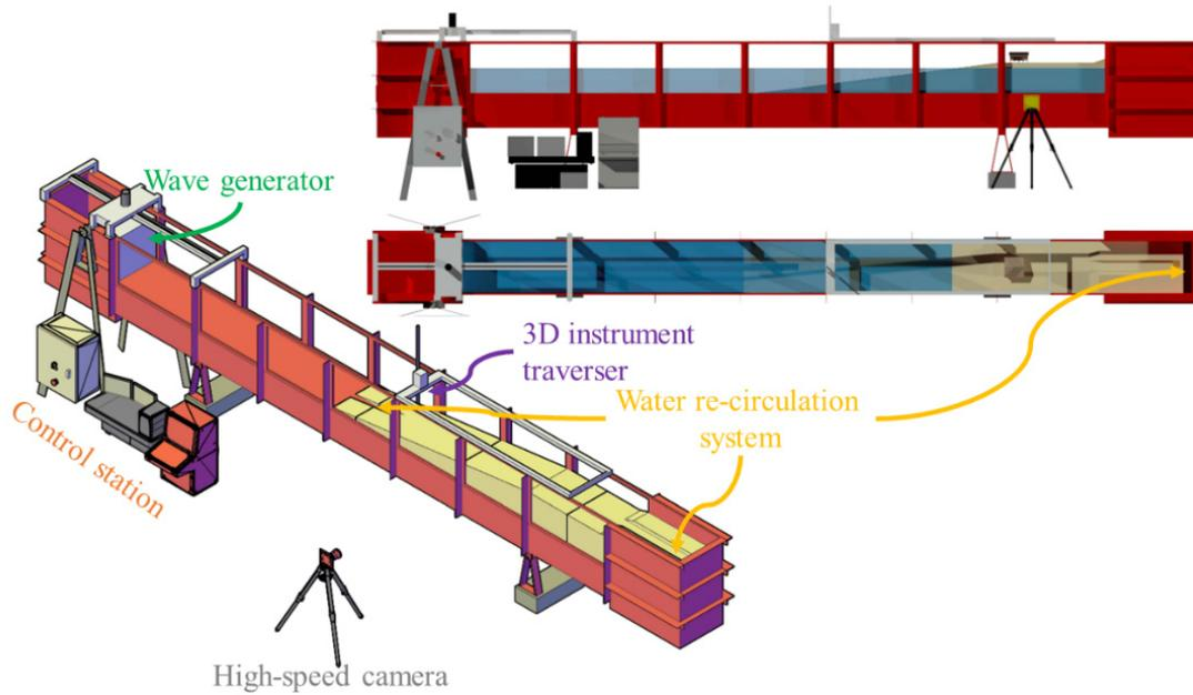
**Figure 7: Wave flume facility at the University of Houston.**
