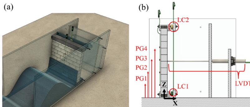
**Figure 8: (a) Orthographic view of the test setup of single masonry walls. (b) Masonry wall instrumentation plan with two load cells (LC1 and LC2), one linear variable differential transformer (LVDT), and five pressure gages (PG1-PG4).**
