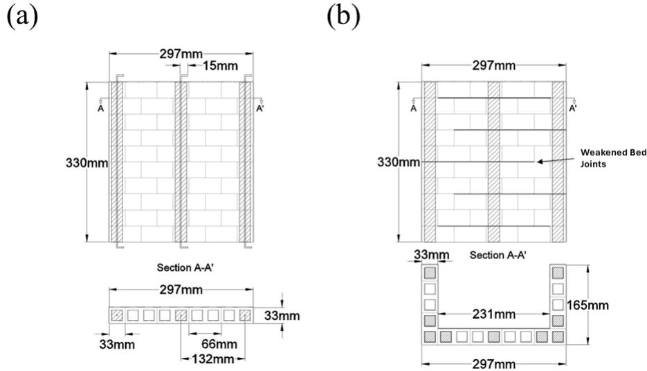
**Figure 6: (a) Schematic of plain Wall-5 and (b) schematic of C-shape Wall-8.**
