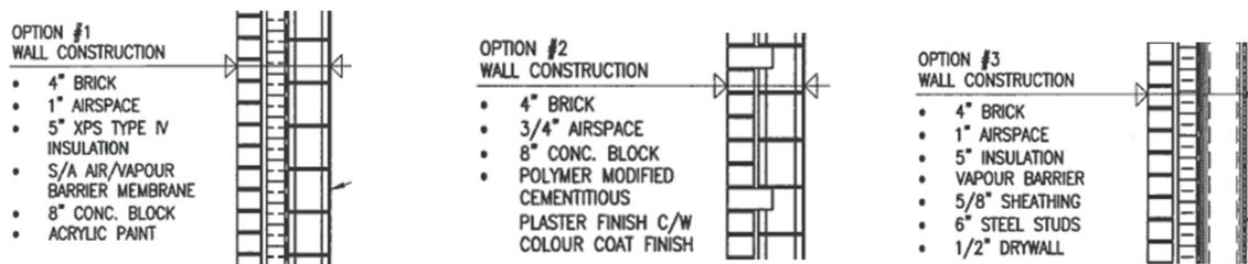
Figure 3: Wall section of hut (1), hut (2) and hut (3).
