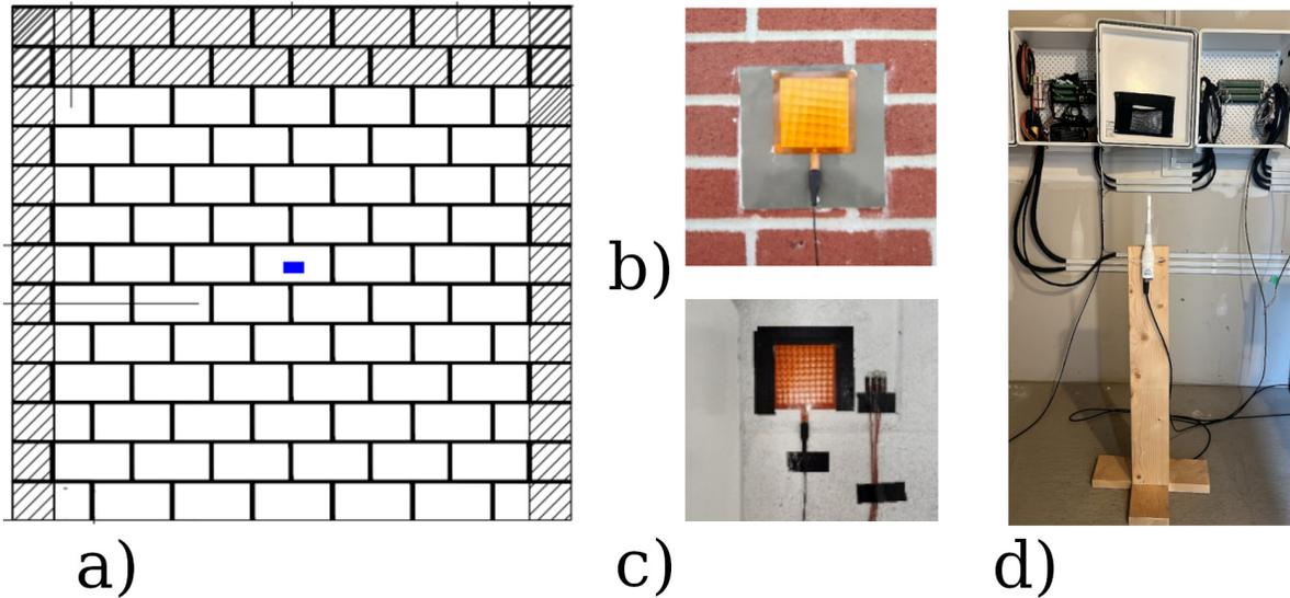
**Figure 2: Sensors and location on walls.**
