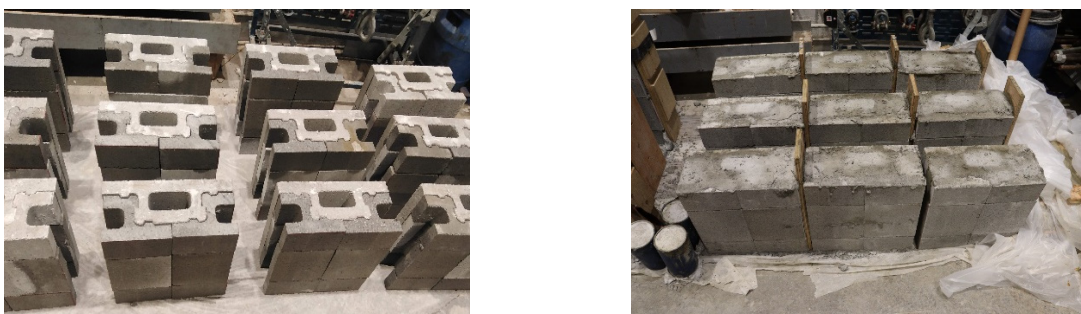
Figure 7: Construction of Sparlock prisms
