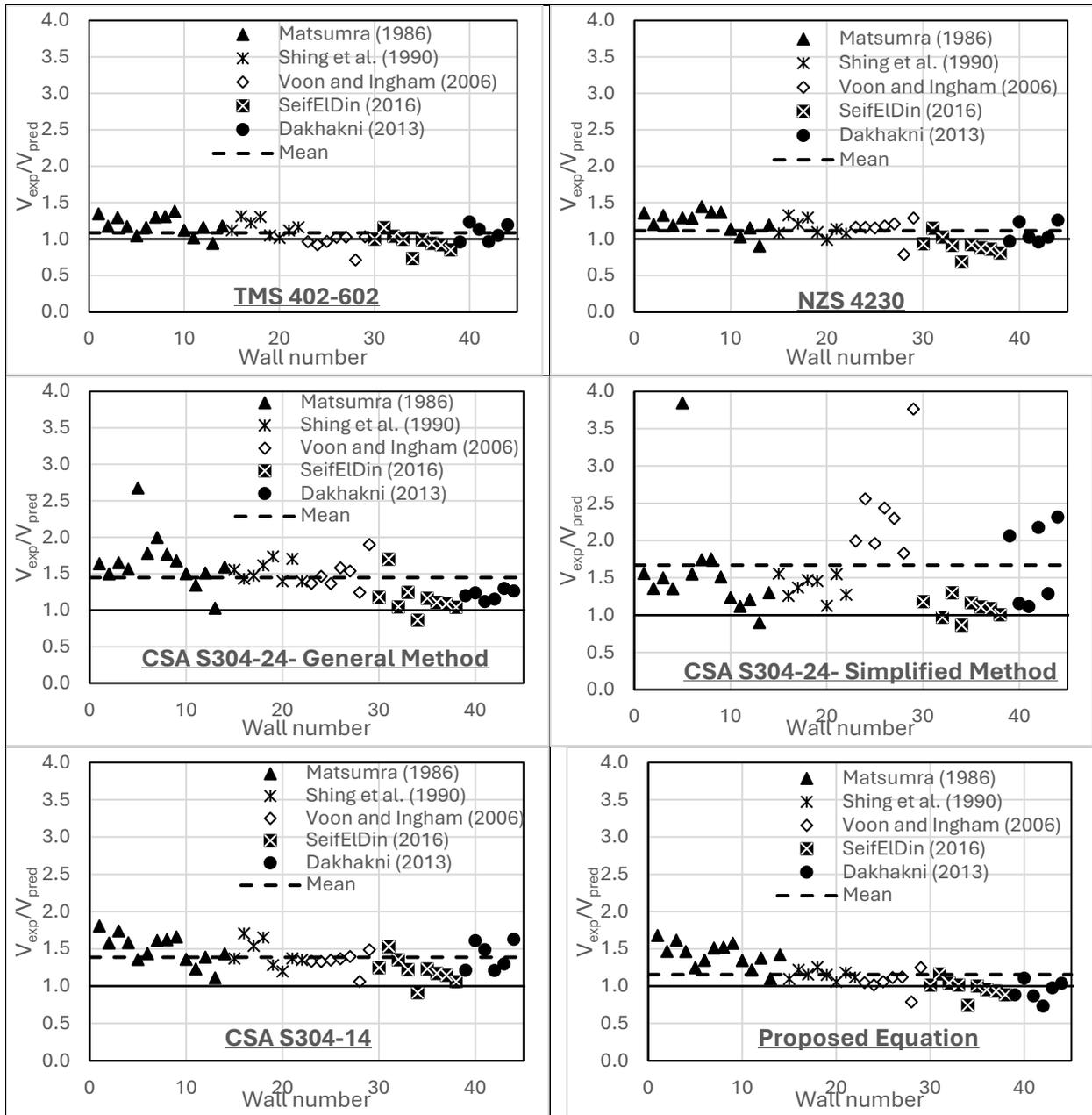
Figure 4:  $V_{Experimental} / V_{Predicted}$  for Shear Design Equations
