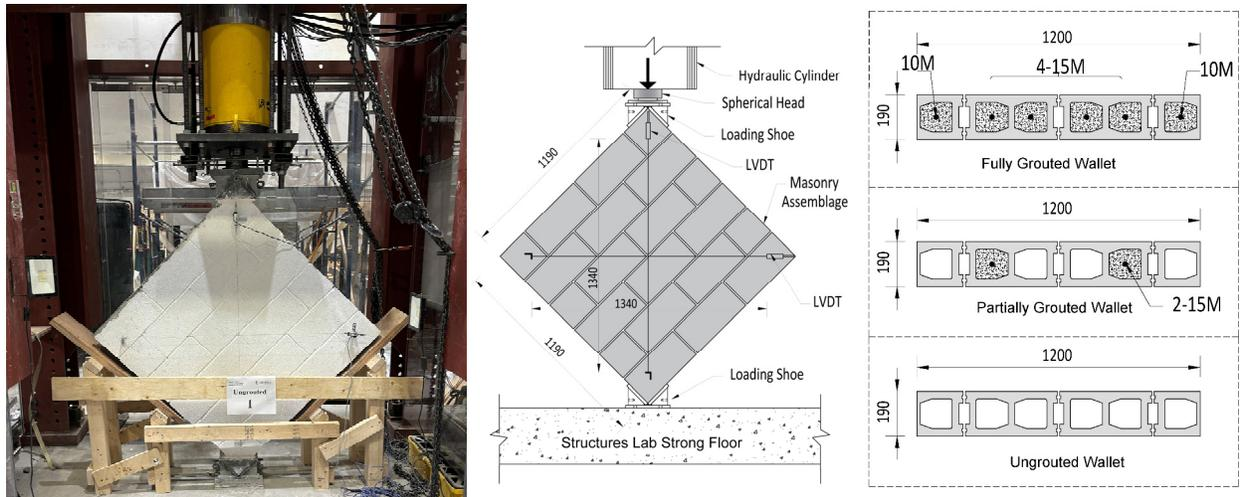
a- Test setup of masonry assemblages
