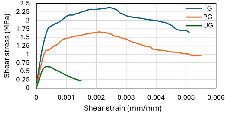
**Figure 3: Average shear stress-strain curves of masonry assemblages**
