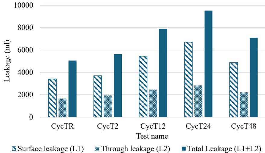
**Figure 3: Comparison of Leakage Amounts Across Different Drying Time Intervals**
