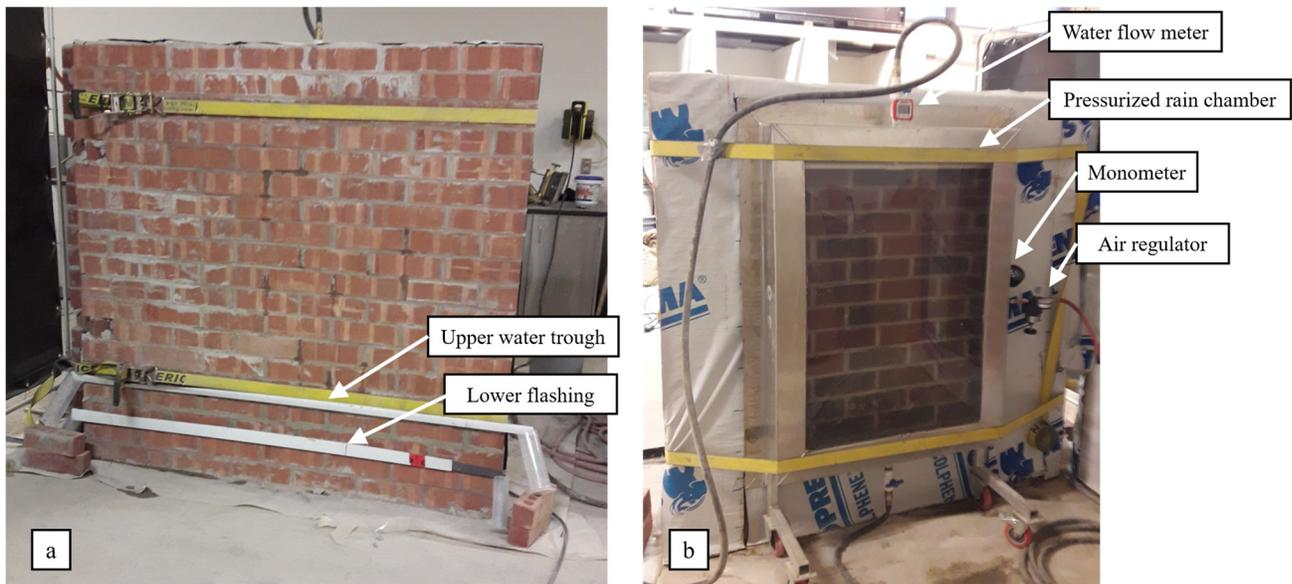
**Figure 1: (a) Upper Water Trough and Lower Flashing Installation on Brick Veneer, and (b) Rain Chamber Setup**
