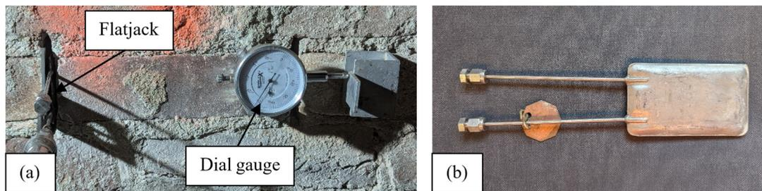
**Figure 6: Flatjack shear testing: (a) test setup and (b) typical flatjack.**
