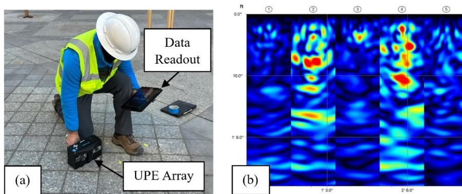
**Figure 2: UPE testing: (a) conducting test and (b) results showing discontinuities in red.**
