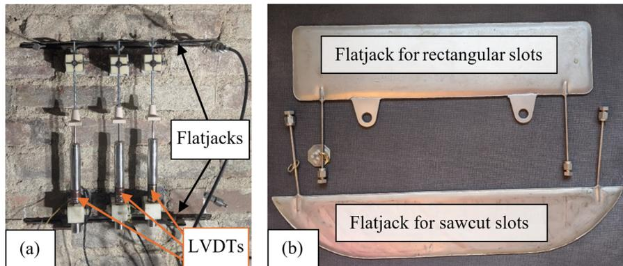
**Figure 5: Flatjack deformability testing: (a) test setup and (b) typical flatjacks.**
