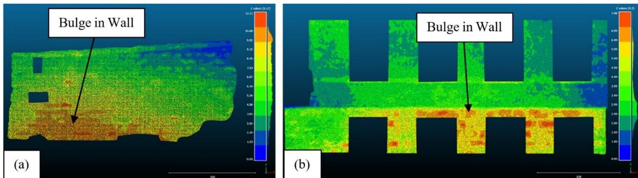
**Figure 1: LiDAR contour plots: (a) of a stone masonry retaining wall and (b) of a brick masonry wall.**
