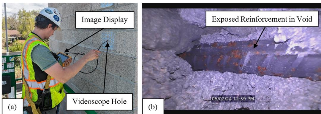
**Figure 3. Videoscope probe: (a) operating videoscope and (b) videoscope image.**
