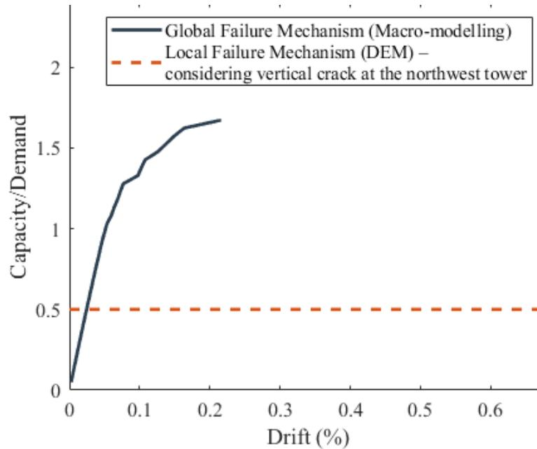
**Figure 9: Capacity/Demand Comparison Between Local and Global Failure.**
