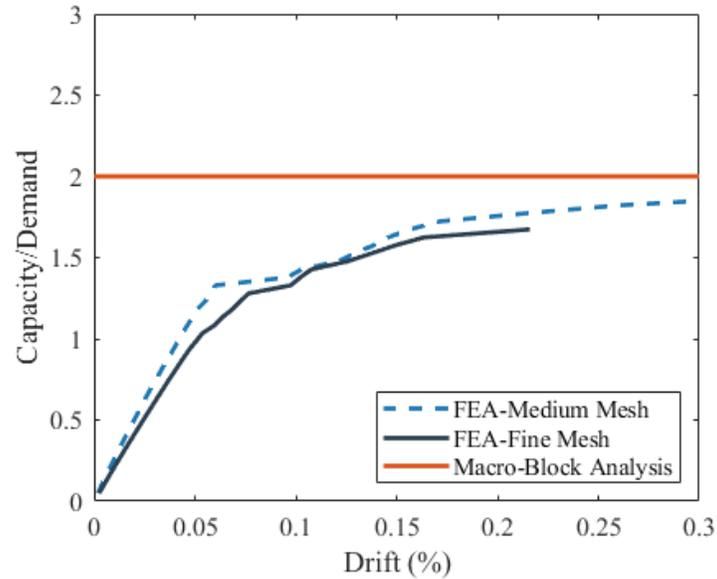
**Figure 6: Capacity/Demand Comparison for Global Failure.**
