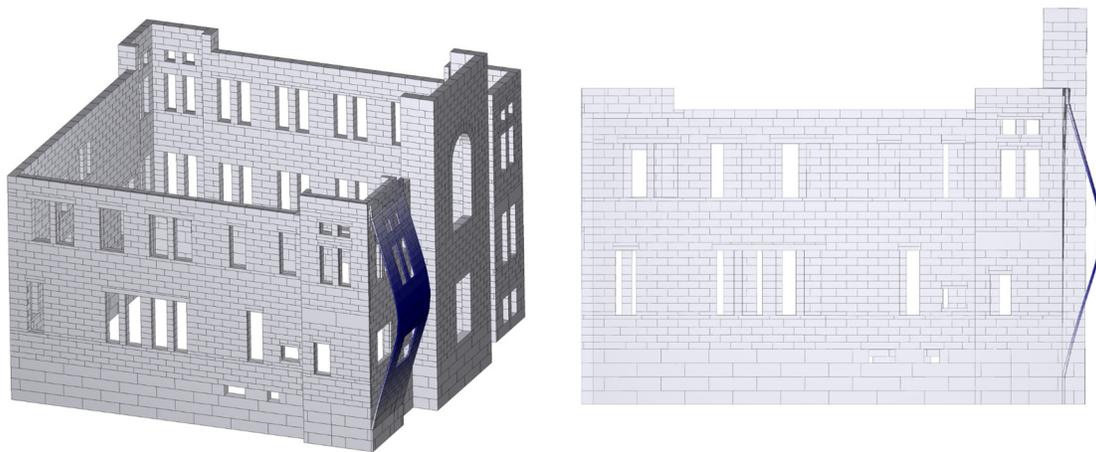
**Figure 8: DEM Model Local Failure Mechanism (Deformation Factor: 5).**
