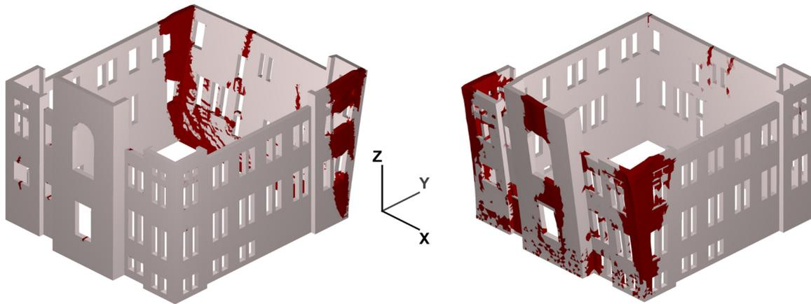
**Figure 3: Continuum Model Failure Mechanism (Deformation Factor: 5), under wind loading applied in the positive Y-direction (left), negative Y-direction (right).**
