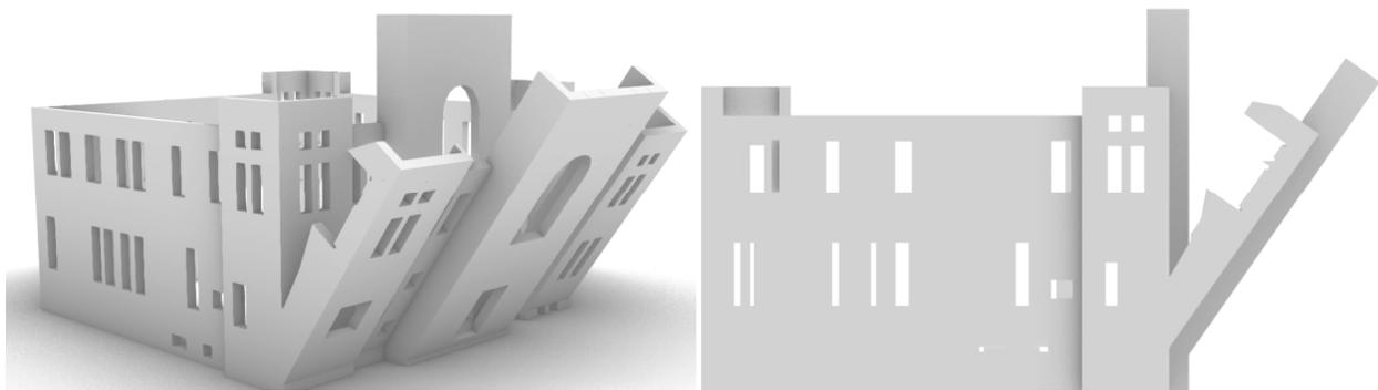
**Figure 5: Macro-blocks and Failure Mechanism for the Overturning of the Front Façade.**
