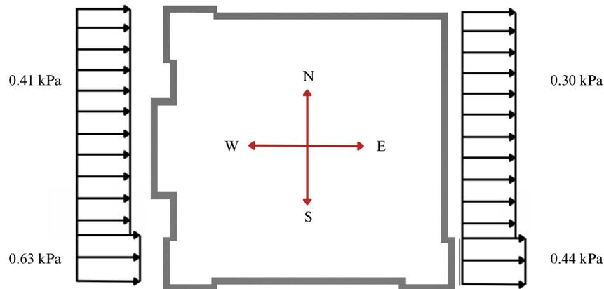
**Figure 2: Wind Loading Profile for Case-Study Building.**
