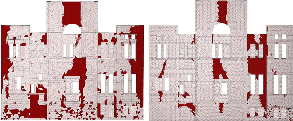
**Figure 4: Plastic Tensile Strain Distribution on the Front Façade for Medium Mesh (left) and Fine Mesh (right) under the applied wind loading in the negative-Y direction.**
