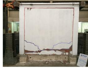
(b) Crack pattern in the infill wall test
