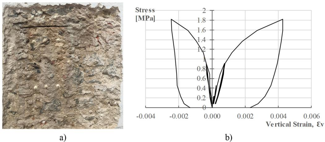
**Figure 4: a) Inspection area, b) stress-strain curves obtained from double flat-jack tests.**
