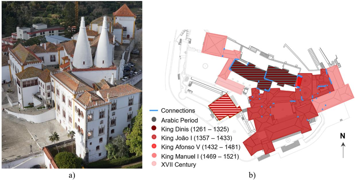
**Figure 1: The National Palace of Sintra, Portugal: a) side view picture, b) plan view with construction timeline and identified connections between buildings**
