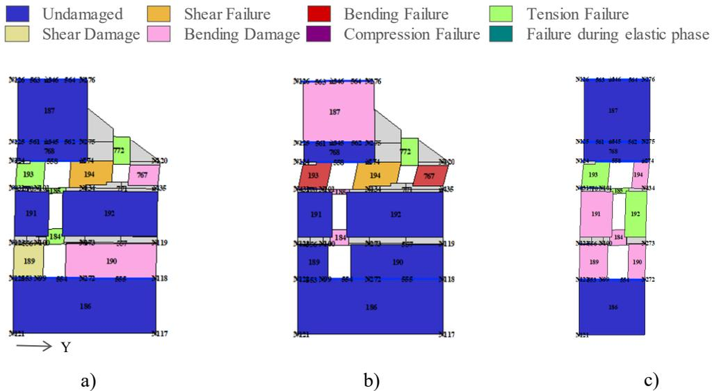
**Figure 8: Damage pattern of wall 19 in the Y direction shared between Unit 1 and Unit 2 for a top wall horizontal displacement of 0.02 m**
