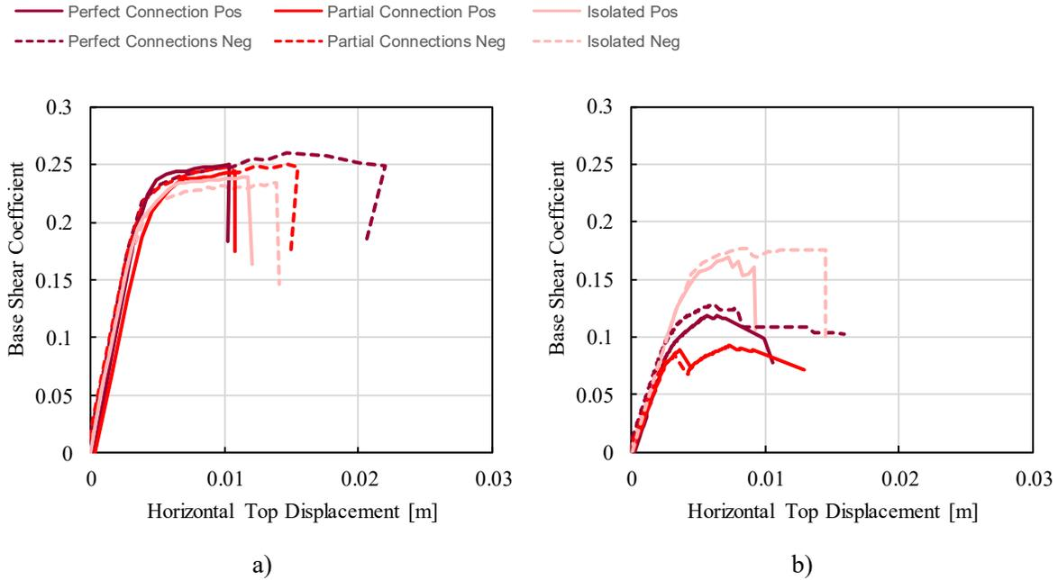
**Figure 7: Pushover curves for Unit 1: a) x direction, b) y direction, considering a uniform loading**
