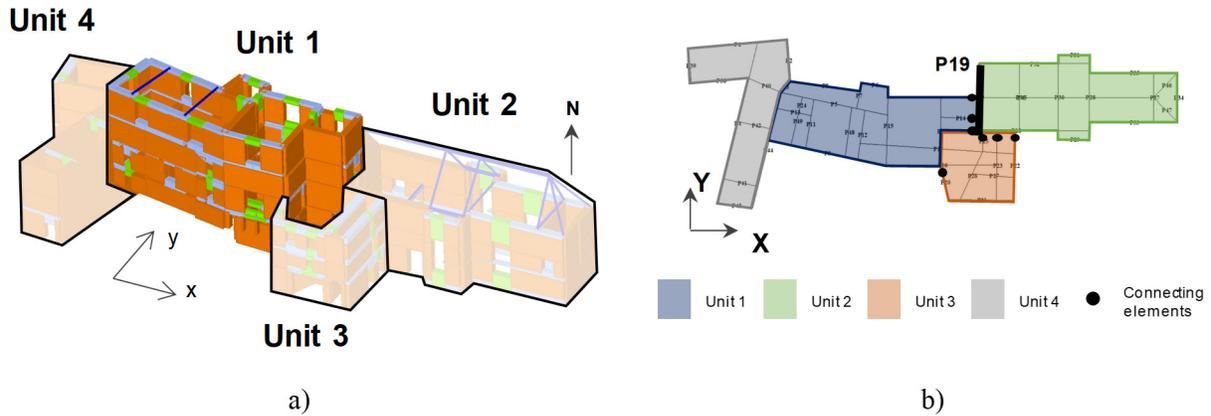
**Figure 6: Numerical model: a) 3D view of the mesh, b) plan of the units and location of connecting elements**
