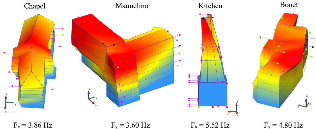
**Figure 5: First frequency and modal shape of the main tested structural units (from [9])**
