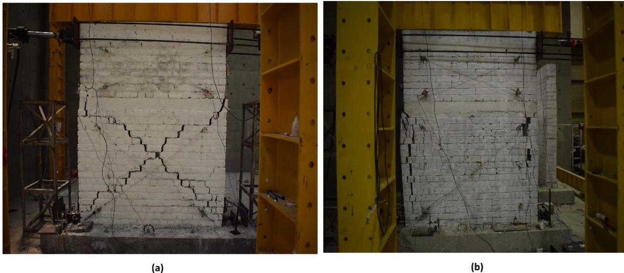
**Fig. 4. Damage pattern after test (a) traditional masonry and (b) ICEB masonry**
