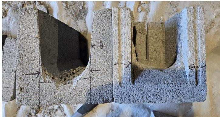
**Fig. 8: Cross sections of lintel unit (left) and knock Out unit (right) used in the test**
