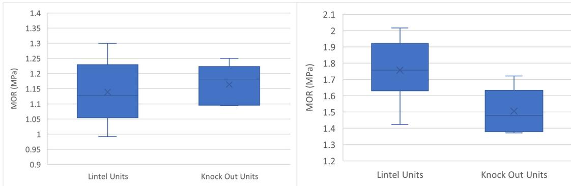
**Fig. 7: MOR values for beams(left) and bond wrench specimens (right) varying block**
