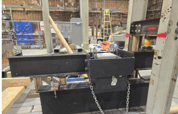
**Fig. 3: Schematic of the bond wrench test set up (left) and physical test set up (right)**
