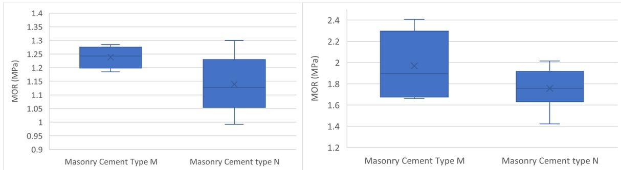
**Fig. 6: MOR values for beams(left) and bond wrench specimens (right) varying Mortar**
