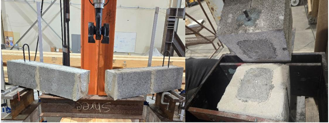
**Fig. 4: Typical failure of beam (left) and bond wrench specimens (right)**
