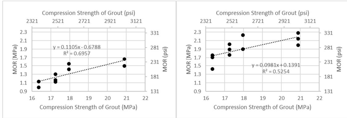
**Fig. 5: MOR values for beams(left) and bond wrench specimens (right) with respect to varying grout strength**
