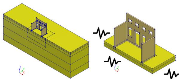
**Figure 8. Model simplification for NLTH Analyses.**
