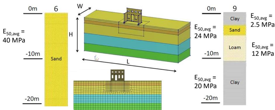
Figure 2: View of the model, symmetrical on the XZ plane, for one type of façade.
