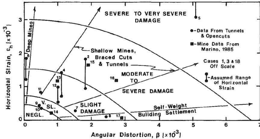
Figure 1: Diagram from Boscardin and Cording [1] with damage predictions at combinations of horizontal strain and angular distortion.
