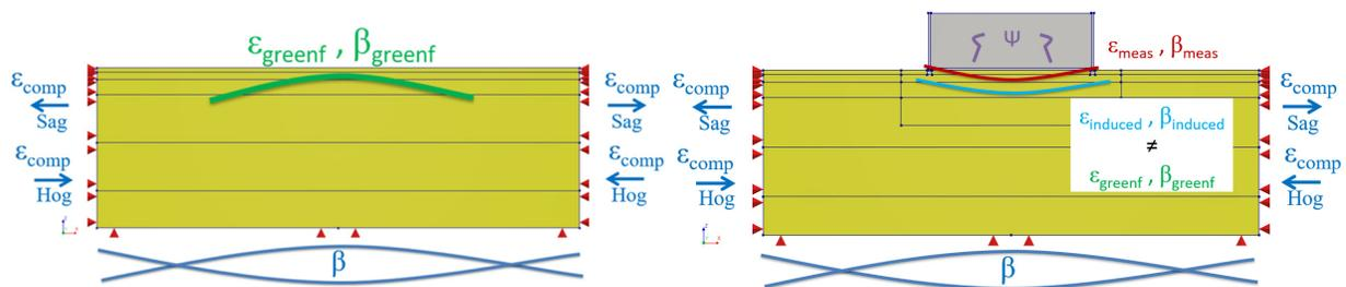
**Figure 3: Two-step model: left, only greenfield, and right, soil+building.**
