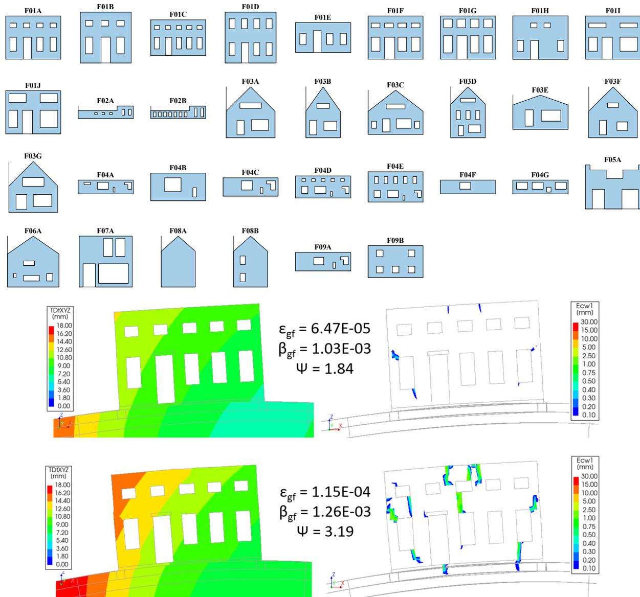
**Figure 4: Variations of façade geometries and deformation of façade F01C subjected to strain/curvature and its measured damage.**
