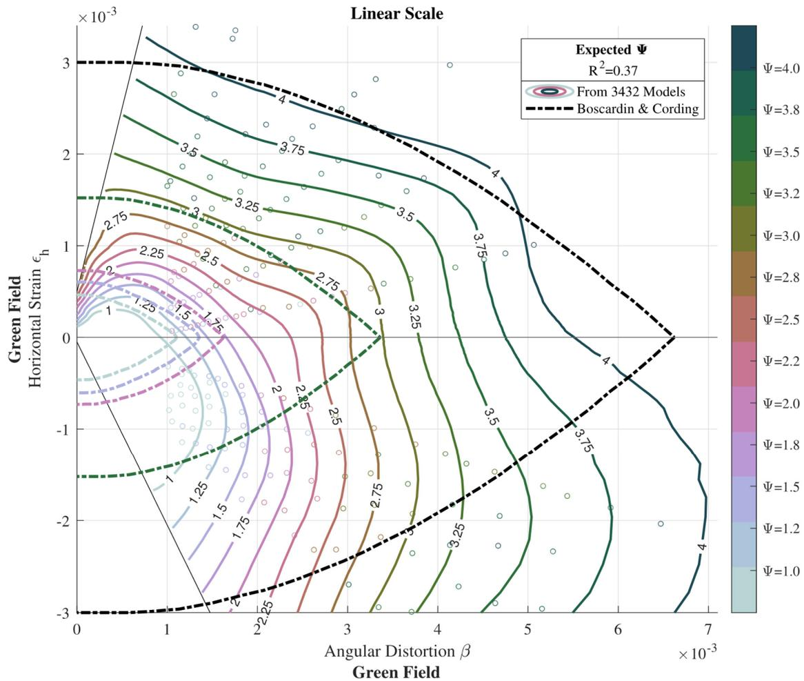
Figure 7. Iso- $\Psi$  contours showing the expected value of  $\Psi$  at combinations of  $\epsilon$  and  $\beta$ .
