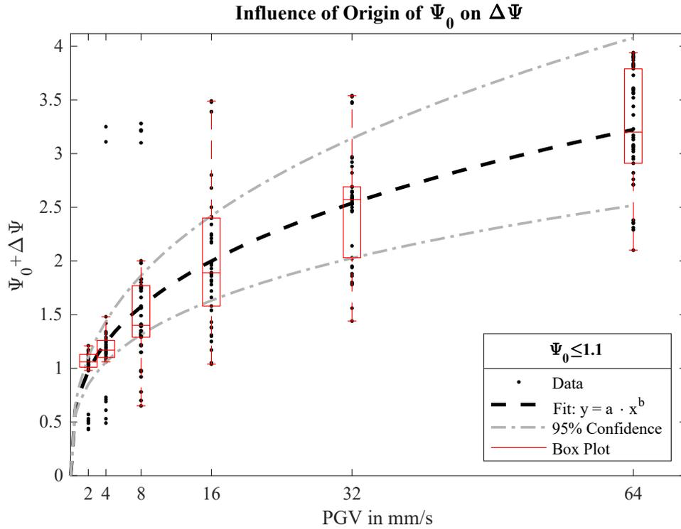
**Figure 9. Increase in damage ( $\Delta\Psi$ ) due to vibrations for various initial values of damage.**
