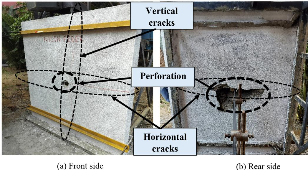
**Figure 10: Damages in Nylon Fibre-Strengthened Wall in the Last Hit.**
