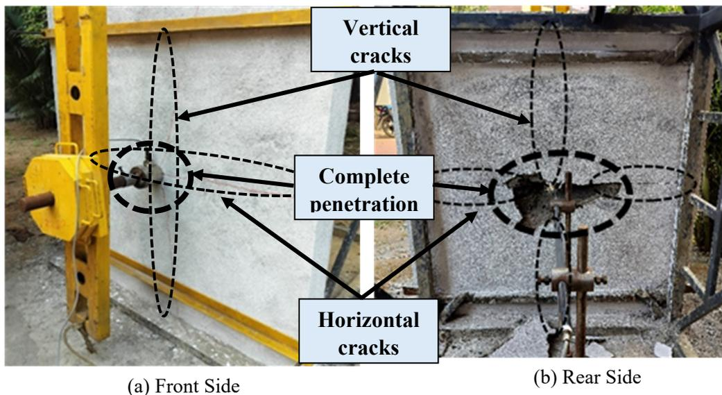
**Figure 6: Damages In URM Wall In the Last Hit.**
