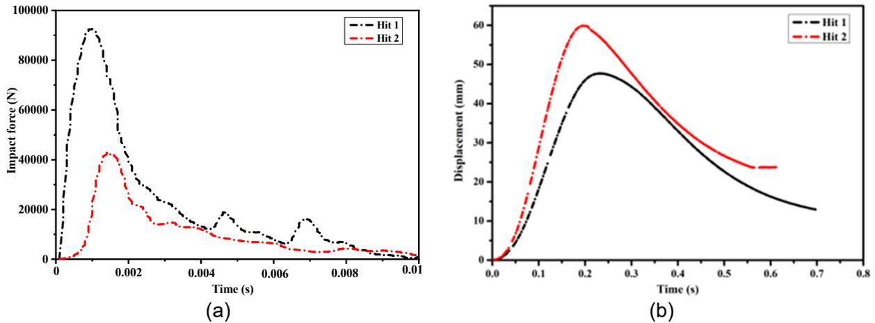
**Figure 5: Impact Loading History of URM Specimen: (a) Force-Time History; (b) Displacement-Time History.**
