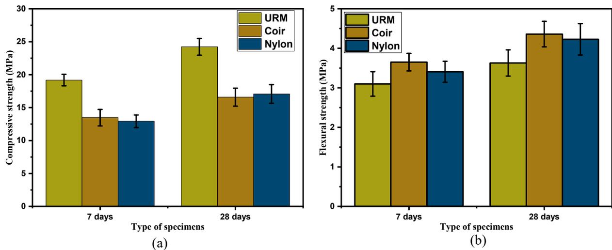
**Figure 3: (a) Variation in Compressive Strength for Unreinforced and Fibre-Reinforced Cubes; (b) Variation in Flexure Strength for Unreinforced and Fibre-Reinforced Prisms.**
