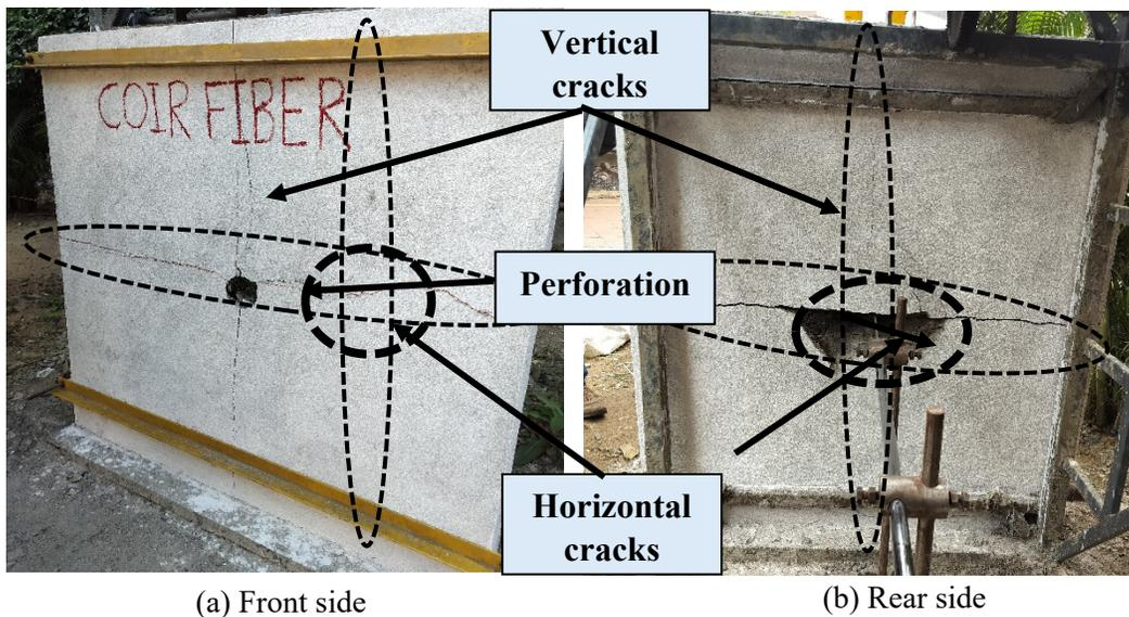
**Figure 8: Damages in Coir Fibre Strengthened Wall in the Last Hit.**
