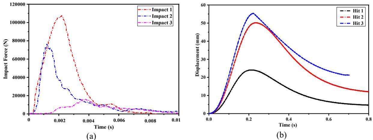
**Figure 9: Impact Loading History of Nylon Fibre-Strengthened Specimen: (a) Force-Time History; (b) Displacement-Time History.**
