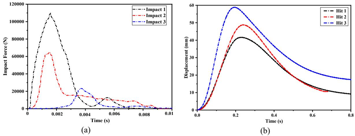
**Figure 7: Impact Loading History of Coir Fibre-Strengthened Specimen: (a) Force-Time History; (b) Displacement-Time History.**
