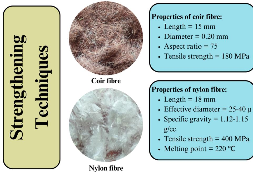
**Figure 2: Physical and Mechanical Properties of Coir and Nylon Fibres.**
