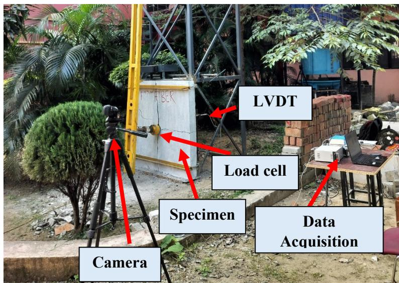
**Figure 4: Impact Loading Test Setup and Instruments.**
