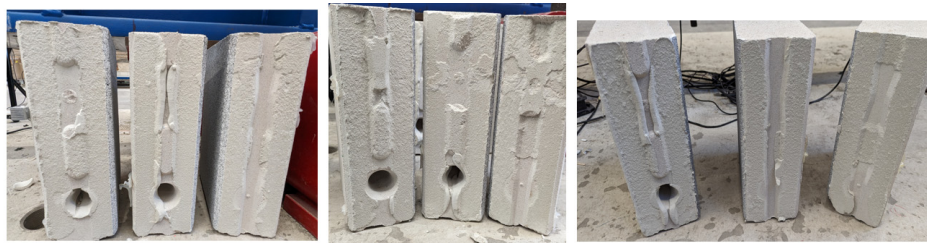
Figure 8: Failure surface in CS-Block.
