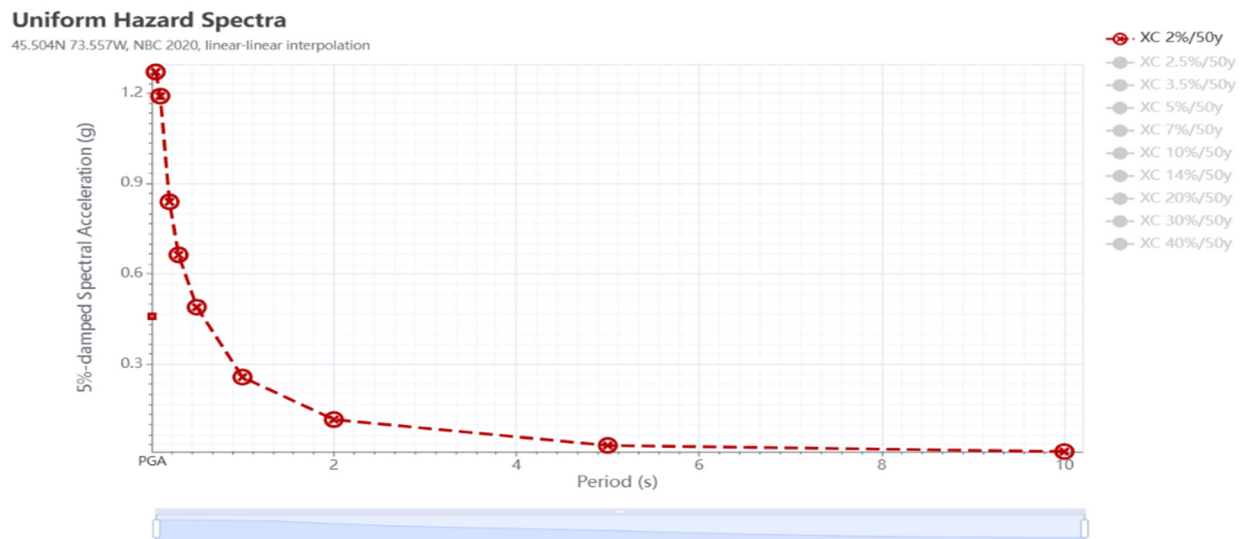
Figure 9: The 2020 Uniform hazard spectrum for site class C in Montreal with a return period of 2% in 50 years
