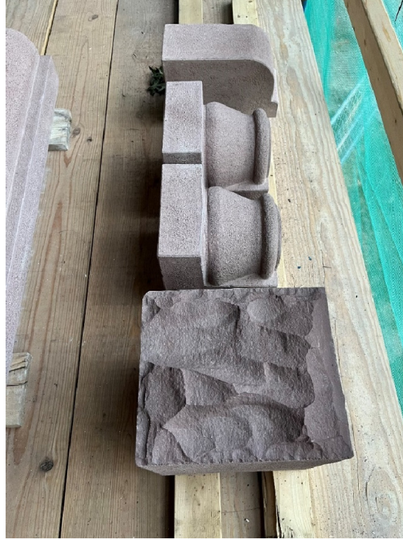
Figure 5: Bush-hammered (top) and quarry-faced (bottom) profile showing color changes from tooling.
