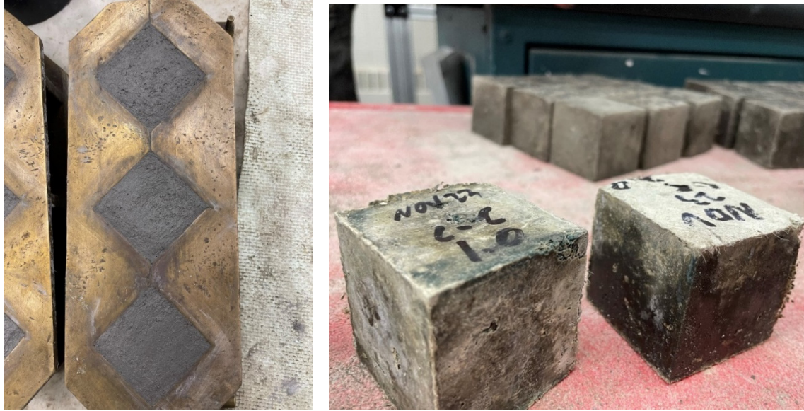
Figure 2: a) Cube moulds for mortar compression tests and b) mortar cubes for compression tests
