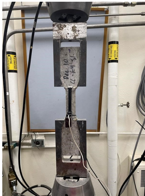
Figure 3: Tensile strength test setup
