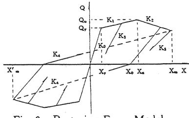
Fig. 3 Restoring Force Model
