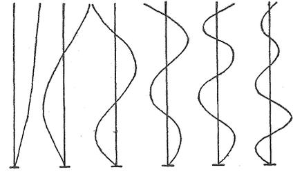
Fig. 5 First 5 Longitudinal Modeshapes
