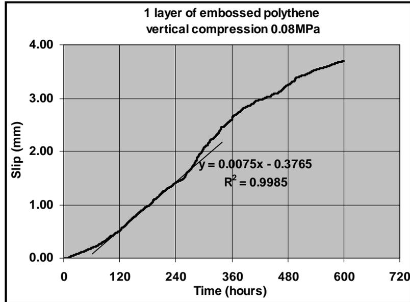
Figure 7. Slip Evolution in Joint Type 3
