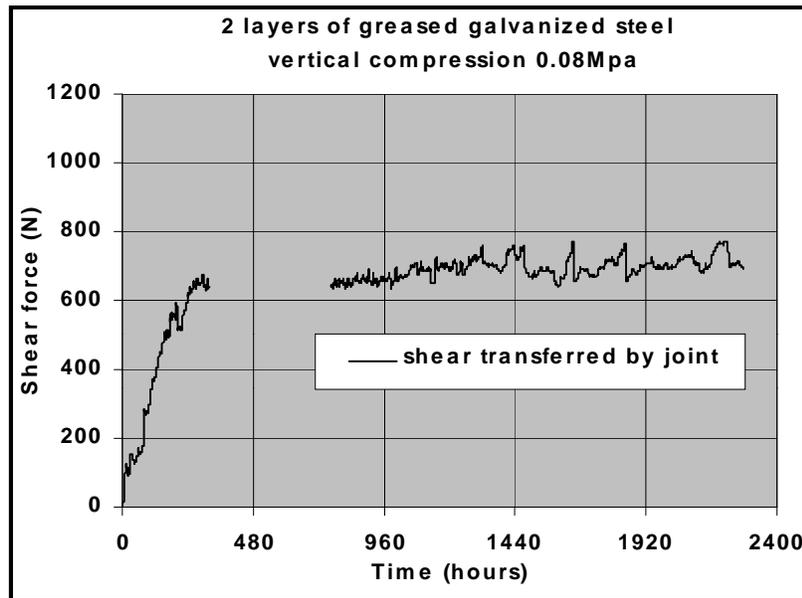
Figure 4. Shear Force Evolution in Joint Type 1
