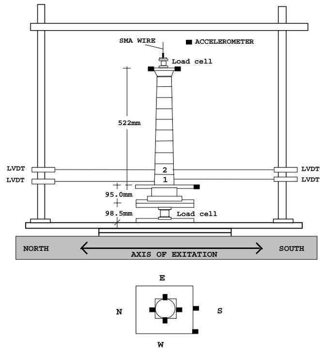
Figure 1b Single steel column on the shaking table
