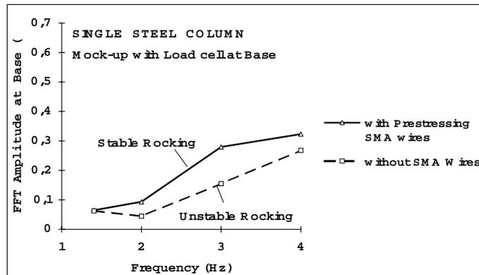
Figure 5b Single column response with and without SMA wires
