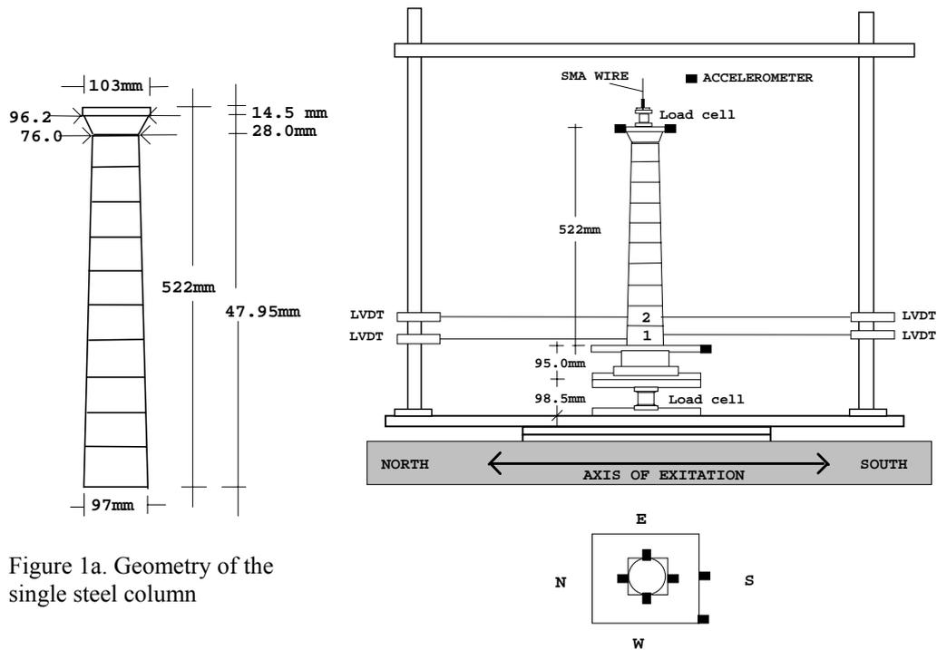
Figure 1a. Geometry of the single steel column
