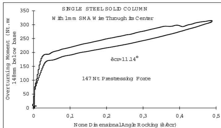
Figure 6b. Static pull-out response of single steel column with SMA wire
