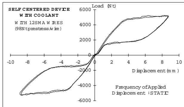
Fig. 4a. SMA Device under “Static” displacement
