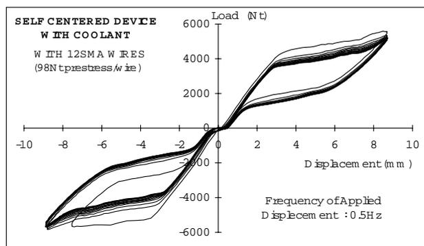
Fig. 4a. SMA Device under “Dynamic” displacement
